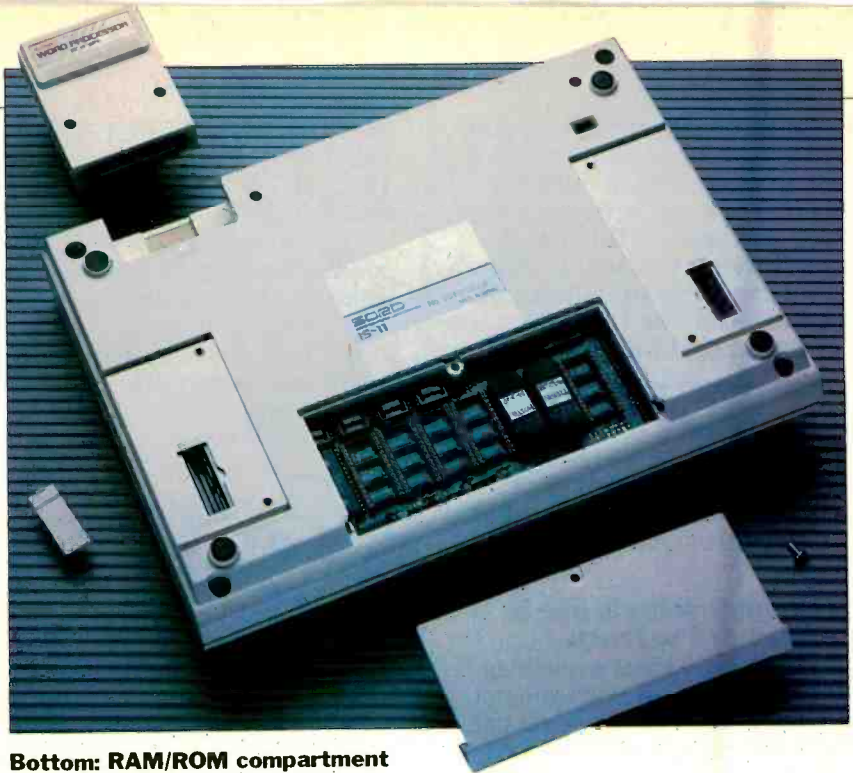
Bottom: RAM/ROM compartment (c), Centronics port (r), keypad port (l), and ROM cartridge (top).
