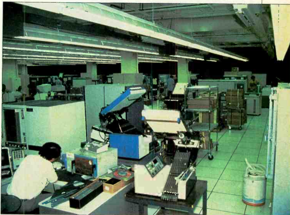
A direct wafer stepping photo-lithography process is used in making the 68020 at Motorola.
