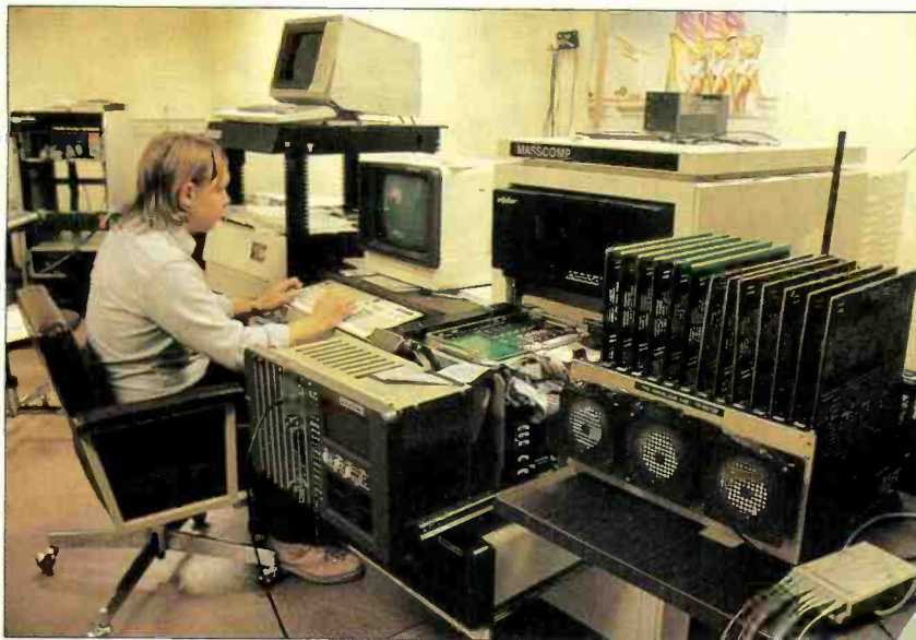
VAT is being developed on a homemade parallel processor 200 times as fast as a Motorola 68000.
