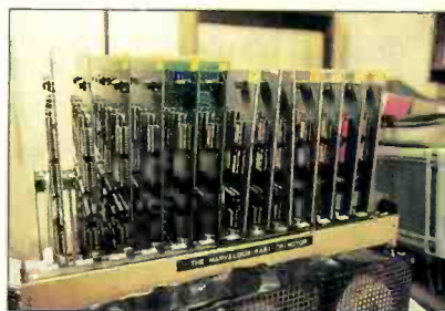
VAT is being developed on a homemade parallel processor 200 times as fast as a Motorola 68000.
