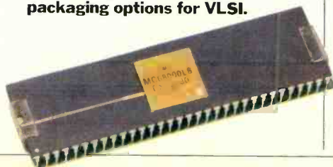
Fig. 4. Some of the proposed packaging options for VLSI.
