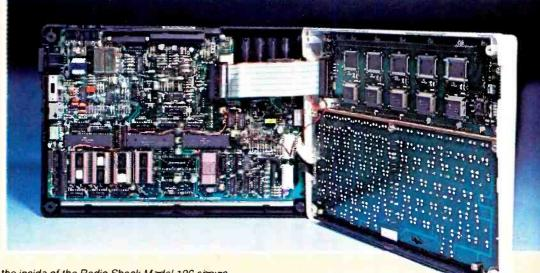
Photo of the inside of the Radio Shack Model 100 shows how compactly and economically the parts are laid out and wired.
