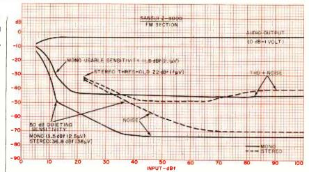
Noise and harmonic distortion for mono and stereo of FM section.
