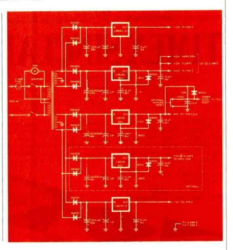
Fig. 19. Schematic of the system power supply.
