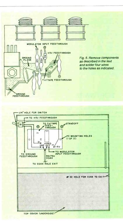
Fig. 6. Position the circuit board and connect the wires as shown here.
