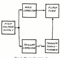
Fig. 1. Block diagram of a flash-tube trigger circuit.
