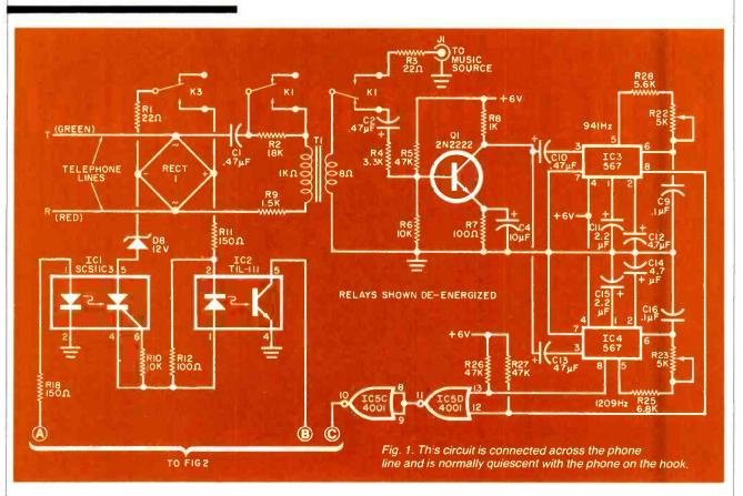
phone to place a caller on hold, any type of phone can be used to return to the caller and remove the hold condition. Power is supplied by a conventional line-operated supply.
