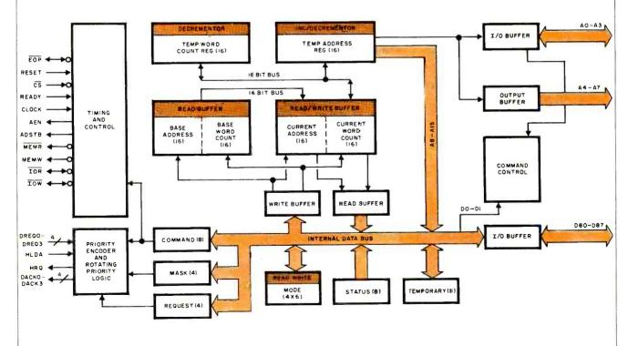
Fig. 20. Block diagram of the 8237A programmable DMA (direct memory access) controller. Connections to it are shown in Fig. 3 in the first part of the series.
