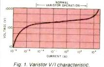
Varistors are primarily used to protect electronic circuits from transient voltage surges. They are particularly useful for protecting computers from power surges that cause memory errors or even loss of memory contents.
