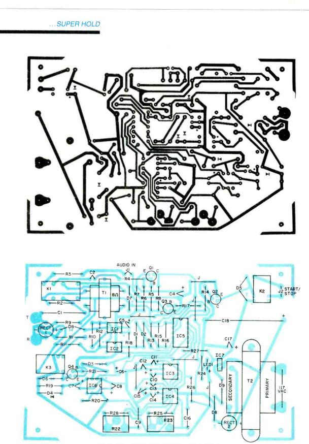
Fig. 3. Same-size foil pattern (top) and component layout for a printed circuit board for the Super Hold.
