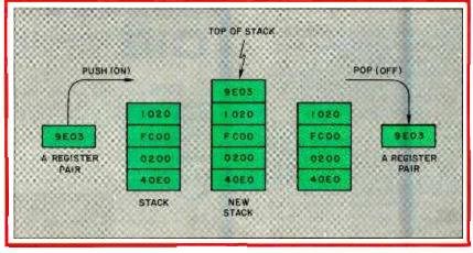
Fig. 4. Stack manipulation.
