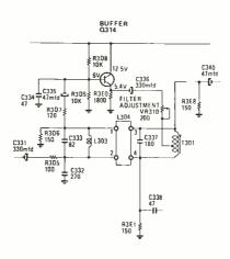
Schematic of the comb filter section of the tuner.
