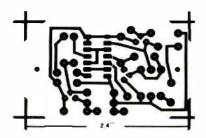
Fig. 3. Foil pattern for the printed circuit board.
