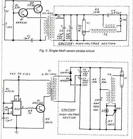
Fig. 4. Xenon strobe flasher circuit.
