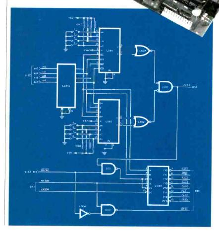
THIS third part of our series on the construction of an 8088based microcomputer compatible with the IBM-PC continues a discussion of the major circuit elements of the system. Also included are schematics of the 64K RAM/ RS232C port board and system power supply (Figs. 13 through 19), which were briefly described in Part 1.
