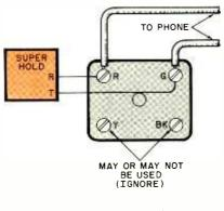
Fig. 4. Use this simple connection while calibrating the Super Hold circuit.
