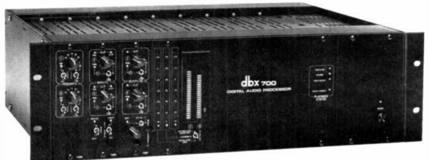
Fig. 1. The dbx Model 700 Digital Processor uses a form of delta modulation instead of PCM.
