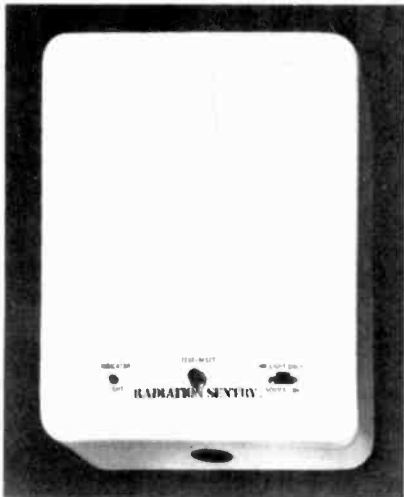
Fig. 2. Wall-mounted Radiation Sentry sounds an alarm at preset level.
