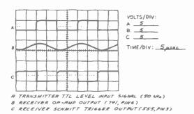
Fig. 8. Received signal waveforms for circuit in Fig. 7.
