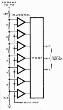
Fig. 2. A 3-bit flash A/D converter.
