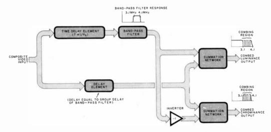
Fig. 8. Comb filter with restricted bandwidth to restore vertical definition.
