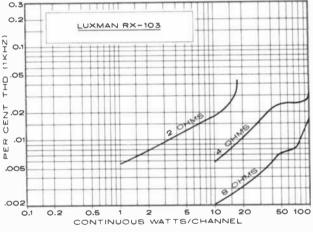
THD at 1000 Hz, both channels driven, left measured.
