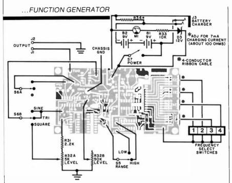
Fig. 6. Connection of off-board components to the pc assembly.
