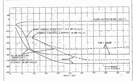
Noise and sensitivity curves for FM section of the RX-103.
