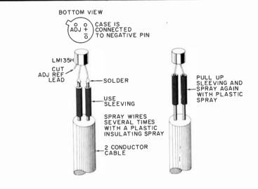
Fig. 8. How to make the sensor assembly.
