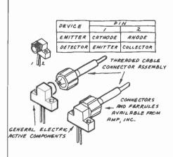
Fig. 1. Construction of GE active fiber-optic components.
