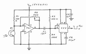
Fig. 7. Fiber-optic receiver with TTL output.
