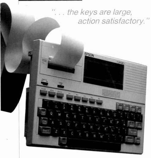
pared to the HP-75C's 10" × 5" × 1¼". But the HX-20 accounts for this most admirably by packing a microprinter and an optional micro-cassette drive or ROM program module easily into its rectangular face.
