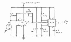
Fig. 9. Fiber-optic receiver with pulse restorer output stage.
