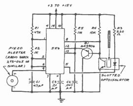
Fig. 2. In a variation of the circuit in Fig. 1, the two 555 timers are replaced by a 556 dual timer as shown here.
