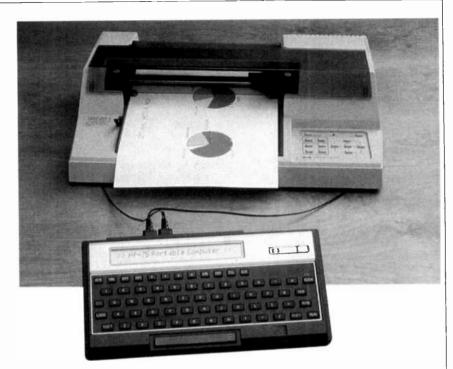
the flexibility to perform as a desktop computer through use of many peripherals presently available and soon to be announced. Unlike handheld computers, its QWERTY keyboard can be used for touch typing, though it does not have the proper-size keys and spacing to satisfy a speed typist.
