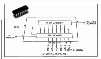
Fig. 3. Ferranti's ZN436 6-bit D/A converter operates from a 5-V supply and has 1-µs conversion speed.
