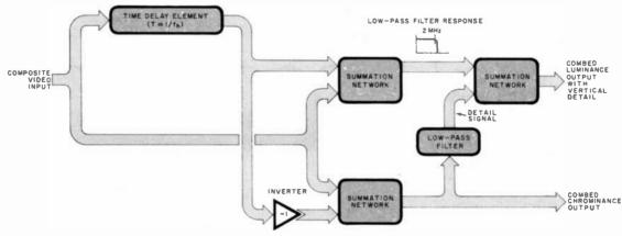
Fig. 9. Adding a "detail signal" to combed luminance output.
