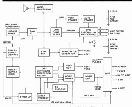
Functional block diagram of the RCA 2023 TV receiver.
