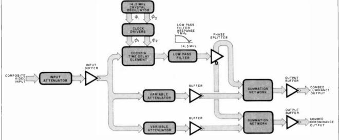
Fig. 7. Block diagram of Fairchild's CCD comb filter.
