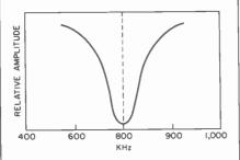
Fig. 1. Frequency characteristic of the notch filter.
