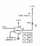
Fig. 3. Basic TTL compatible LED driver.
