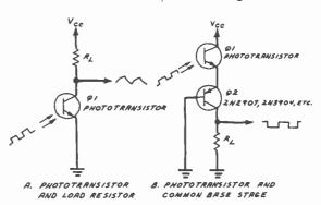
Fig. 5. Two phototransistor circuits.
