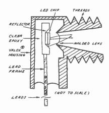
Fig. 2. Internal view of GE side-looking emitter.
