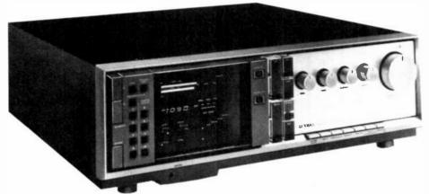
THE Luxman RX-103 AM/FM stereo receiver has digitally synthesized AM and FM tuners and a rated audio output of 90 watts per channel into 8-ohm loads from 20 to 20,000 Hz with no more than 0.018% total harmonic distortion. It features a novel "Servo-Panel" that encloses the front-panel knobs when the set is off, and is retracted by a motor to expose them (together with some pushbutton controls) when it is turned on.
