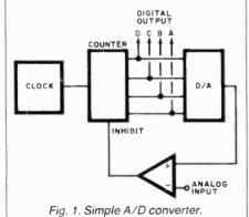
equal, the comparator changes states and inhibits the clock. The binary output from the counter is the digital equivalent of the analog input signal.
