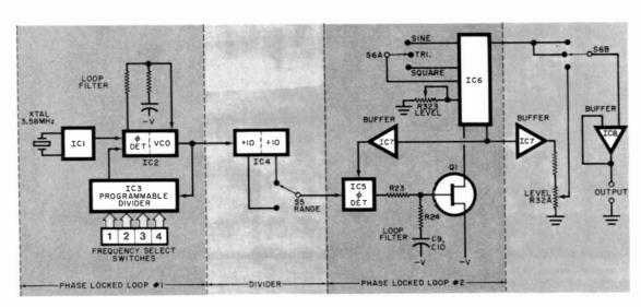
Fig. 1. The basic circuit consists of two phase-locked loops.
