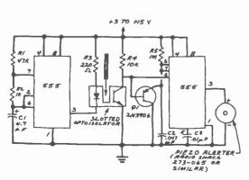
Fig. 1. Schematic of a simple photonic door and window intrusion alarm. Components shown provide a pulsating output tone.
