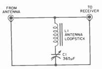
Fig. 2. Schematic diagram of the filter.
