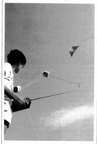
This  $3' \times 6'$  kite can tow a 12-oz RC disc camera package to an altitude approaching 1000 ft.
