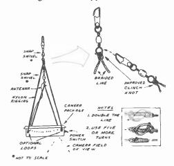
Fig. 4. Rigging the airborne camera package.
