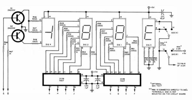
Fig. 4. Schematic of the display circuit.
