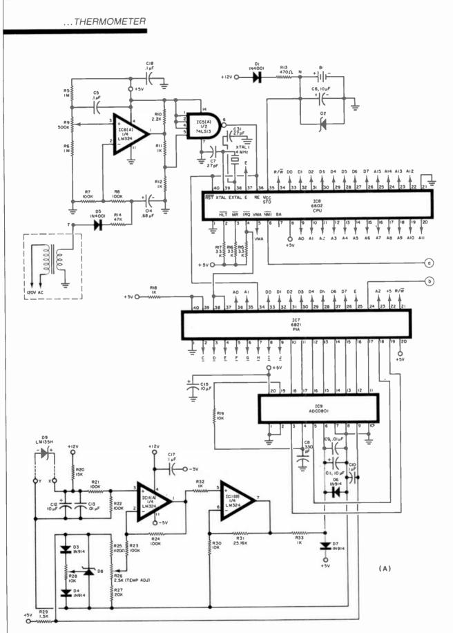
Fig. 3A. Microprocessor and PIA portions of the circuit.
