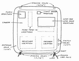
Fig. 3. Bottom view of camera package.
