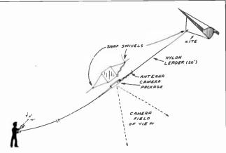
Fig. 5. Taking an oblique-away photo from kite. Variations of this four-line rigging can be attached to a kite line to provide vertical and two kinds of oblique photos. It's also well suited for use with balloons.
