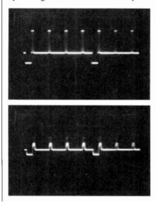
Fig. 1. Color-bar signal: input (top) and output (bottom).
