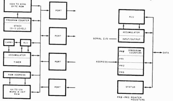
Fig. 1. Block diagram of the AMI S2000 series.
