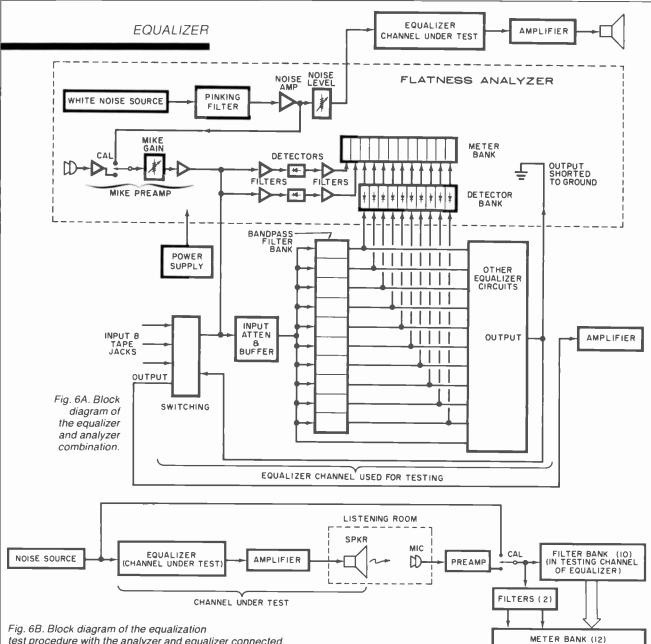
test procedure with the analyzer and equalizer connected.
