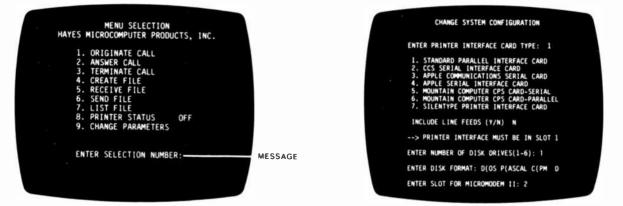
Fig. 2. When the system is ready and booted, the Hayes Terminal Program displays this menu.
