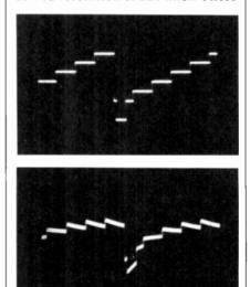
Fig. 2. Staircase signal: input (top) and output (bottom).
