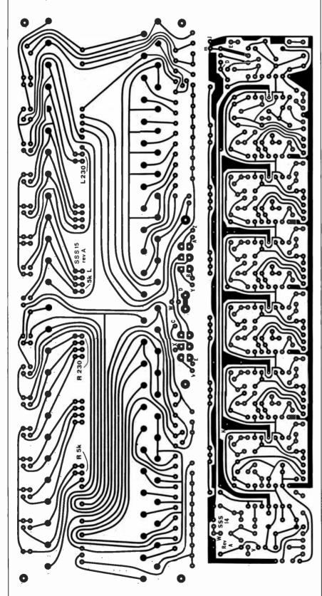
Fig. 3. Foil patterns for the Equalizer pc boards
