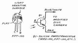
Fig. 4. Light-sensitive trigger for modified camera.
