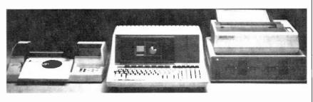
Complete HP-87 system with plotter, disk drive and printer.
