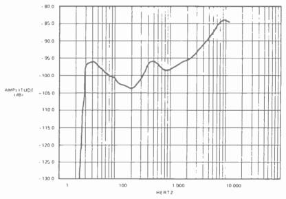
Fig. 4. Equalization curve to be used on response.
