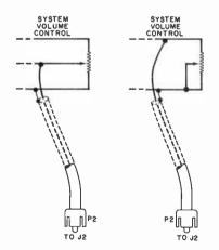
Fig. 2. Connect a shielded cable to the system volume control.
