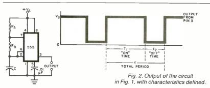
Fig. 1. Standard 555 square-wave generator.
