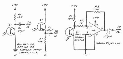
Fig. 2. Phototransistor inputs for 3-digit event counter.
