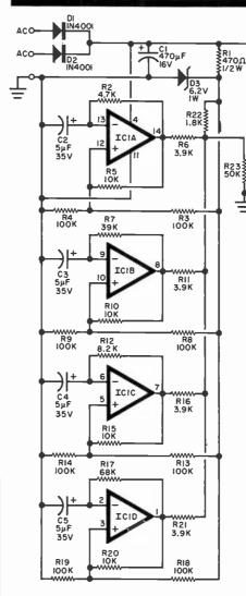
Fig. 2. Four square waves of different frequencies are generated in the four op amps and combined to produce the pseudo-random flicker voltage.
