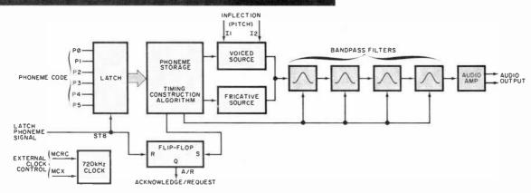
The Votrax SC-01 speech synthesizer chip used in this project is a phoneme type. It contains two voicing generators (voiced and fricative), four speech bandpass filters, a clock generator (710-kHz optimum), and a low-level audio amplifier. There are 64 stored phonemes in seven categories—the first six cover voiced, fricatives, and nasal sounds, while the seventh is silence.
