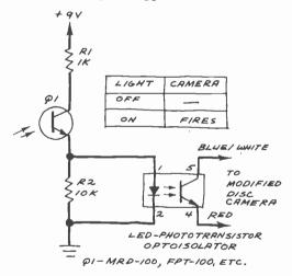
Fig. 5. Improved light-sensitive trigger.
