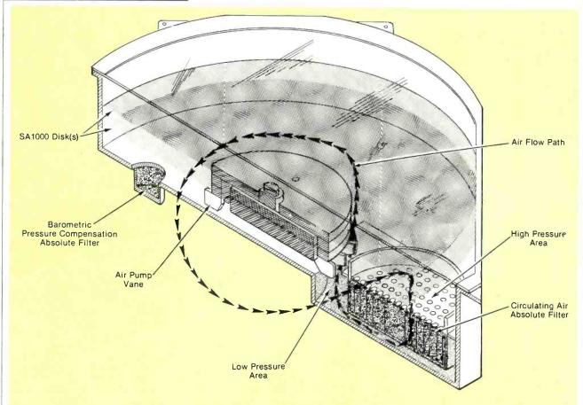
Fig. 1. Air flow diagram of the Shugart SA1000 8" fixed disk system.
