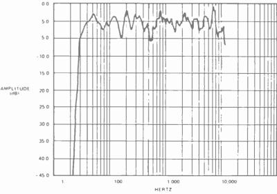
Fig. 5. Response of car with equalization applied
