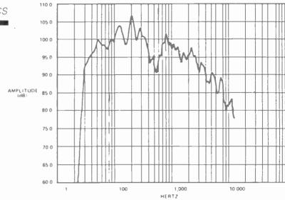
Fig. 3. Response measured in a car without equalization
