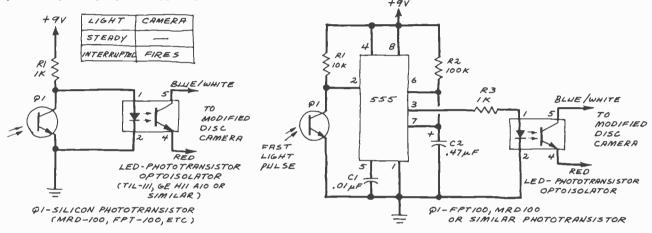
Fig. 7. Trigger activated by a xenon strobe.
