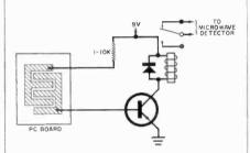
low. Connect the two wires to a pc board that has an interleaved pattern. Mount the board on an angle. When it rains, the wires will conduct, turn the transistor on, and energize the relay.
