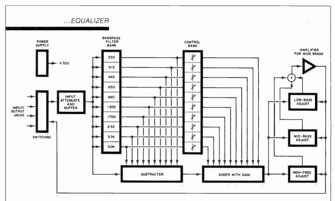
Fig. 1. Block diagram of the Equalizer. Midband frequency selection is made by filter bank.
