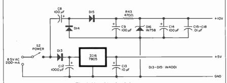
Fig. 6. Use this circuit for a power supply to drive the Speak-Easy speech board.
