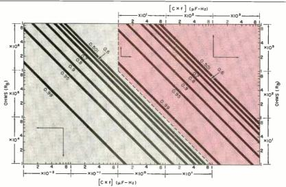
Fig. 3. Plot of  $C \times f$  vs.  $R_s$  which can be used with Fig. 4 to determine circuit values.
