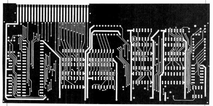
Fig. 6. Foil patterns for the double-sided printed circuit board.
