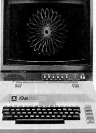
Sound. An ATARI computer has four sound generators, or voices, activated by a separate microchip. This leaves the principal microprocessor chips free to perform other tasks. And you can take full advantage of this capability which is designed for easy programming.
