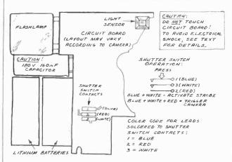
Fig. 5. Connecting leads to the shutter switch terminals.
