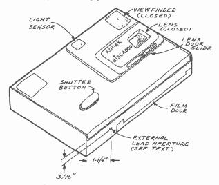
Fig. 4. Location of external leads aperture.
