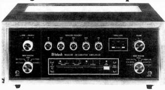
THE McIntosh MA6200 integrated amplifier, rated at 75 watts per channel into 8-ohm loads (or 100 watts into 4 ohms), features the company's exclusive Power Guard circuit that makes it impossible to clip the output waveform. The amplifier can drive up to three pairs of speakers simultaneously, and has control facilities for two tape decks.
