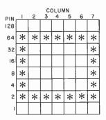
Fig. 4. Converting a shape to numbers.
