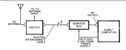
Fig. 8. Use this diagram to connect the automatic switch to the TV and the adapter box and game/computer.
