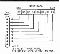
Fig. 3. Relationship between input data and print wires.
