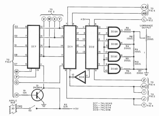
Fig. 5. Luminance output is obtained from D/A IC13.
