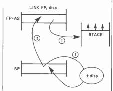
Fig. 3. How the LINK basic instruction is implemented.
