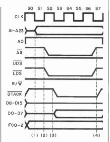
Fig. 5. Timing diagram of a byte read cycle.
