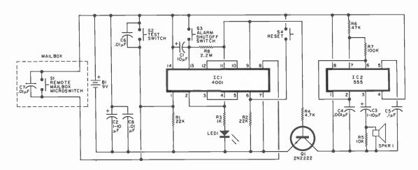
Fig. 1. Heart of the circuit is the 4001 chip set up as a dual set-reset latch.
