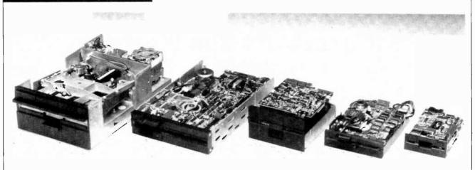
The shrinking world of disk drives is shown by a conventional 8" at left, followed by a half-size 8", conventional and half-size 51/4", and 31/2" drive at far right.
