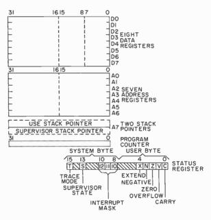
Fig. 1. Programming model of the 68000 microprocessor.
