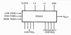
Fig. 2. External connections to R5620 Universal Active Filter.
