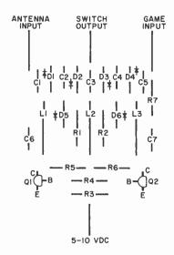
Fig. 5. Component layout for pc board.
