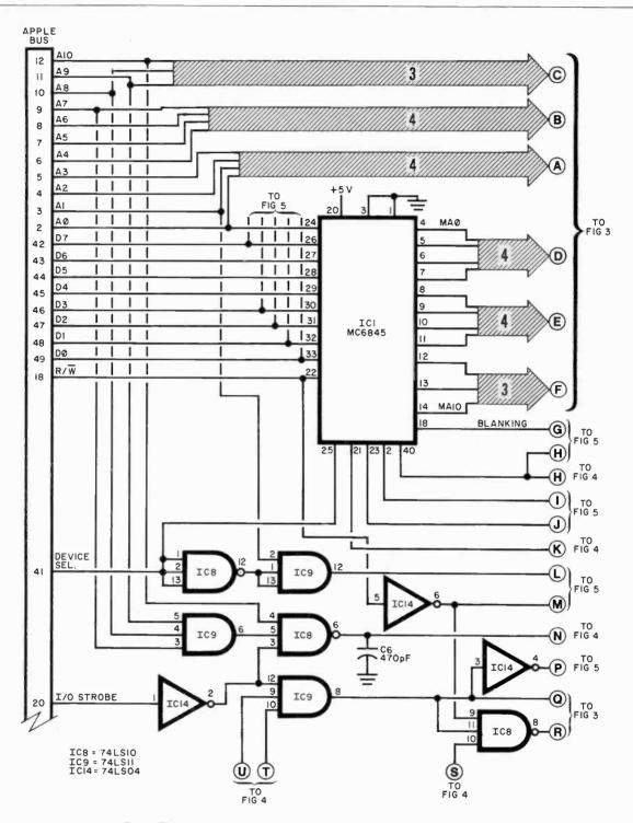
Fig. 2. The 6845 synchronously regenerates the video RAM addressing.
