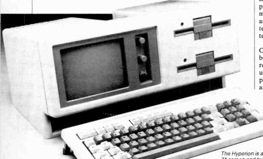
The Hyperion is a 20-lb portable with 7" screen and two 5¼" disk drives which run PCDOS.
