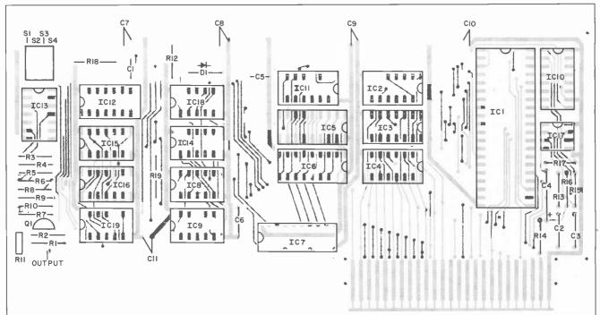
Fig. 7. Component layout for the printed circuit board.
