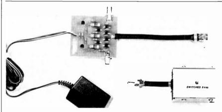
Photo showing the automatic switch, adapter box, and power converter.
