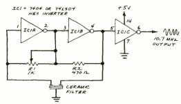
Fig. 6. Schematic diagram of a 10.7-MHz ceramic oscillator.
