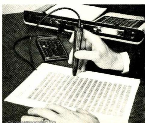
Programs and data can be loaded into the HP-41 via the keyboard or with the help of a handheld wand that reads bar code. The wand permits lengthy listings to be loaded quickly and error free. Barcode listings are supplied with HP-41 software. A service for converting commonly used programs into bar code is available.
