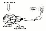
Fig. 1. Flashing a neon lamp with a crystal microphone element.
