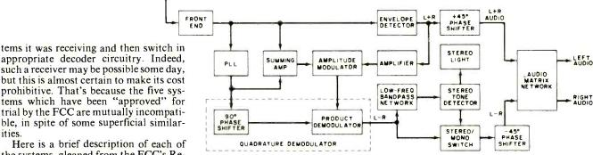
Fig. 3. Single-receiver diagram for Kahn/Hazeltine ISB system.
