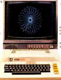
Sound. An ATARI computer has four sound generators, or voices, activated by a separate microchip. This leaves the principal microprocessor chips free to perform other tasks. And you can take full advantage of this capability which is designed for easy programming.
