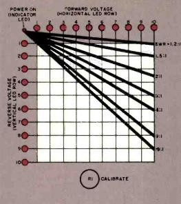
Fig. 2. The display consists of a simple grid whose horizontal (forward voltage) and vertical (reverse voltage) axes are studded with LEDs.
