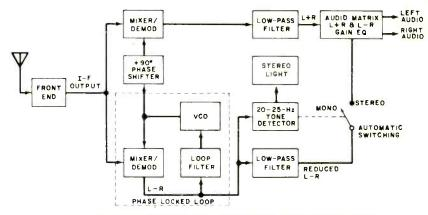
Fig. 2. Basic configuration of an early version of the Harris system.
