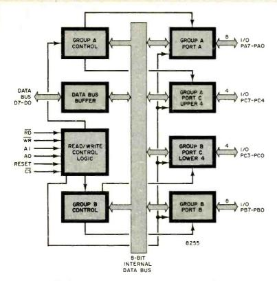
Fig. 4. Internal logic arrangement of the Intel 8255A.
