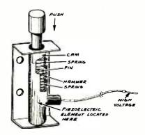
Fig. 2. Vernitron 3652 piezoelectric high-voltage pushbutton.
