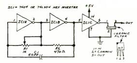
Fig. 3. Test circuit for a ceramic filter.
