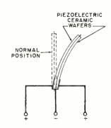
Fig. 2. Piezoelectric bimorph.
