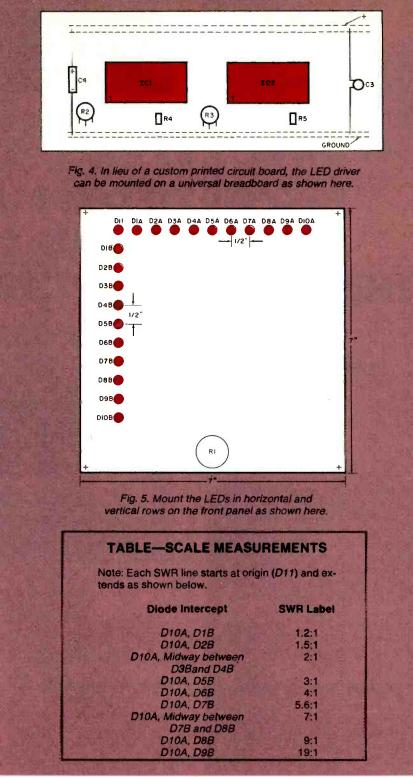
ing D9A lit instead of D10A). This keeps the circuit from saturating. Now note which diode in the vertical column is lit, and read the SWR from the calibration line closest to the intersection extrapolated from the lit diodes. For example, if D10A is lit in the horizontal row and D5B is lit in the vertical row, the intersection lies on the 3:1 SWR calibration line.
