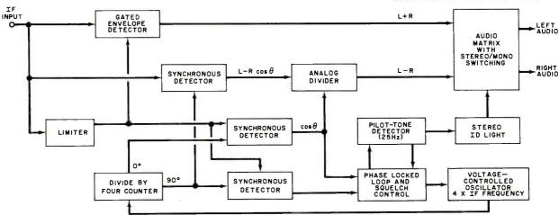
Fig. 5. Block diagram of stereo AM decoder for Motorola C-QUAM system.
