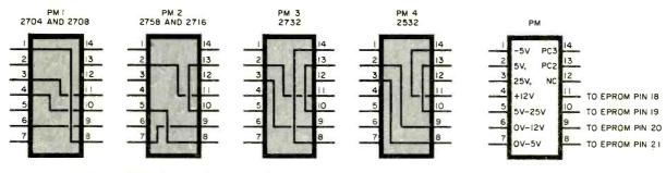
Fig. 6. Wiring diagrams for personality modules to accommodate the various types of EPROMS.
