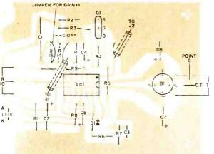
Fig. 2. Use the foil pattern at top to make a printed circuit board and install components as shown.
