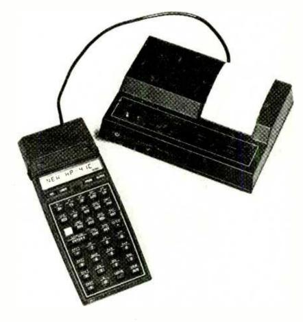
The HP-41C shown here is generating the function sine x. The output, with the curve, is shown on the printer.
