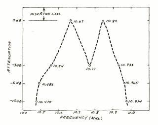
Fig. 5. Measured bandpass of a 10.7-MHz ceramic filter.
