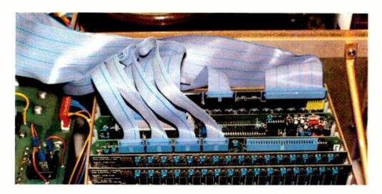
Using an 8-slot motherboard, a hard-disk controller is combined with a floppy controller having DMA capability.
