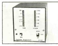
The new M-827 from Palomar Engineers is designed to compute standing wave ratios automatically and display them on a light bar. SWR reading is claimed to be accurate regardless of input power level (which is also displayed on a light bar adjacent to the SWR display). The M-827 has a frequency range rated at 1 to 30 MHz and power range of 20, 200, and 2000 W. The SWR scale is 1 to 10, with logarithmic response. \$98.
