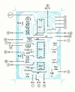
Fig. 4. Component placement diagram.
