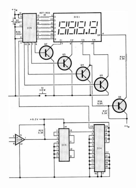
S1, S2—Normally open, momentary-contact pushbutton switch
