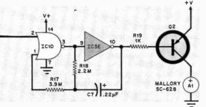
Fig. 2. The circuit in the project uses a CMOS phase-locked loop to detect the presence of the alert signal. The CMOS components cause little battery drain so that the monitor can be in use constantly.
