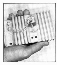
Fig. 7. A DH laser with collimating
