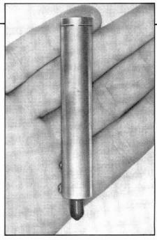
Fig. 6. A battery-driven miniaturized single-heterojunction laser transmitter.
