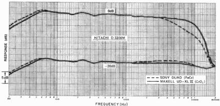
Frequency-response curves for four different types of tape.
