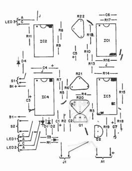
er than soldering them directly to the board. This makes replacement of defective ICs infinitely easier and eliminates the possibility of damaging them during soldering. Be sure to observe polarities and pin basings when you mount the diodes, transistors, LEDs, ICs, and electrolytic capacitors.
