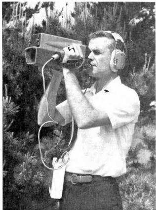
Fig. 4. A long-range laser communicator made by American Laser Systems.
