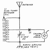
Fig. 1. Super-simple diode AM radio.
