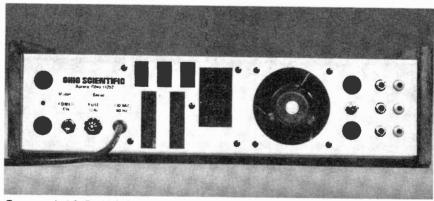
Rear panel of C4P with I/O ports.
