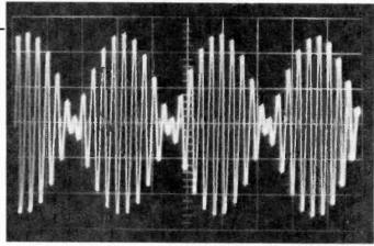
Fig. 1. Oscilloscope photo of the alert signal of the Emergency Broadcast System. It consists of two tones at 853 Hz and 960 Hz broadcast for 22.5 seconds.
