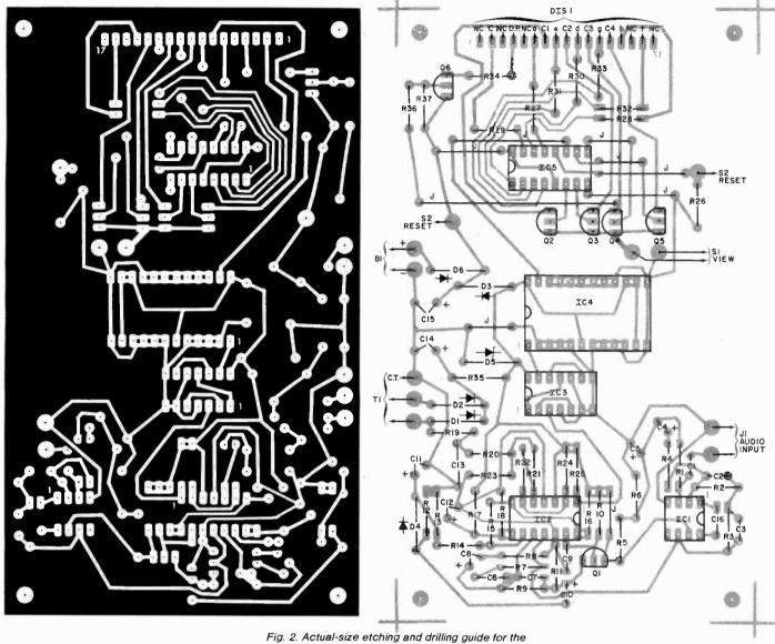
Fig. 2. Actual-size etching and drilling guide for the printed circuit board is above left, component layout at right.
