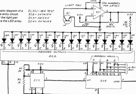
address of the selected LED will then appear on the 4-bit bus between IC2 and IC4.
