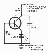
Fig. 5. Simple pulse driving circuit for injection laser.
