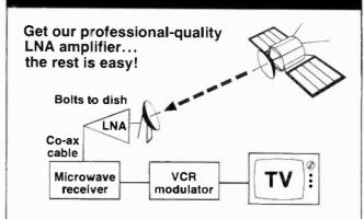
The only sophisticated component you need is a low-noise amplifier to boost the satellite signal.
