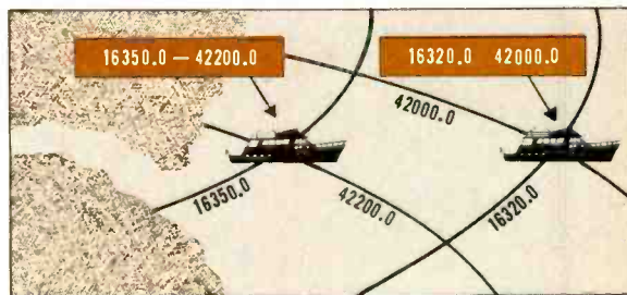
Fig. 2. Radiolocation by LORAN-C signals and charts. A special receiver directs the user to two curved "lines of position." The intersection of these lines pinpoints receiver location.
