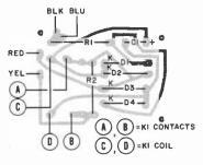
Fig. 2. Actual-size etching and drilling guide, right; component placement above.
