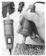
and lead hole cleaning, among other jobs. It runs at about 9000 rpm and accommodates drills and burrs with shank size up to 1/4". Less than 5" long (excluding drill bit), the Iso-Tip is small enough to use at close quarters. The device is housed in high-impact plastic and is equipped with a 10' power cord, as well as a collet chuck, four collets and two drill bits.
