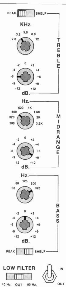
plication is yet another equalizer referred to by many as the "console type." Virtually all professional mixing consoles use this sort of device, with one available for each mike or line input. Additional equalizers are often devoted to echo and reverb lines.
