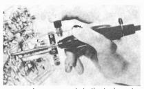
means of compressed air, the tool creates suction in its tip, with the high-pressure air flow causing a continuous self-cleaning action as well. Air can be supplied either from a pressurized line or by an ordinary foot pump. The tool has a tip 2.4 mm in diameter with a 1.2-mm vent. \$39.95.
