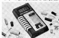
ing for stray capacitance of test leads. Measurements appear on a 0.5" (12.7mm) high liquid crystal display. An internal fuse prevents instrument damage from charged capacitors and should the test leads be inadvertently connected across a voltage source. Uses a single 9-volt alkaline battery. \$149.00
