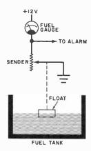
Fig. 1. Typical fuel-gauge circuit.
