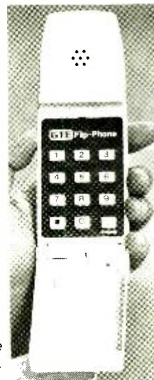
The Flip-Phone flips open to reveal the keyboard and the privacy switch.
