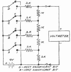
Fig. 4. D/A demonstrator circuit.
