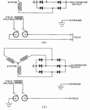
Fig. 3. Three types of alternators found in automobiles: floating field (A); pulled-up field (B); grounded field (C).
