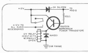
Fig. 8. Relay circuit for remote control of booster amplifier.
