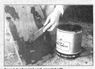
Sound-deadening board, secured with roofing cement, suppresses rattles and resonances which may occur with sheet-metal door panels.
