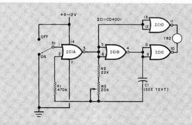
Fig. 2. This ultrasonic transmitter employs four NOR gates.
