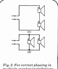
Fig. 2. For correct phasing in multiple-speaker installations, wire "unlike" terminals in series as at (A), "like" ones in parallel as at (B).
