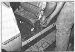
Unscrewing carpet-retaining plate provides handy channel for wires feeding signals to amplifiers or to the rear speakers.
