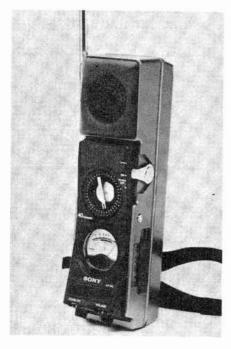
he hand-held Model ICB-1020 AM transceiver from Sony uses the latest in phase-locked-loop (PLL) synthesizers to provide coverage on all 40 CB channels. It is powered by eight AA cells that fit within its housing and has provisions for obtaining power from a 12-volt mobile electrical system and, with an adapter, standard 117-volt ac line power. Whichever power source is used, the rated r-f output power from the transmitter is 1 watt.
