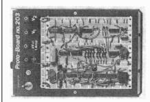
provide additional power and signal connections. The power supply is rated at 1 A,  $5 \pm 0.25$  V, with 10 mV combined ripple and noise at  $\frac{1}{2}$  A out, and is protected against short circuits. Dimensions are  $6\frac{1}{2}$  x  $9\frac{3}{4}$  x  $3\frac{1}{4}$  in. (16.5 x 24.8 x 8.3 cm), \$80.
