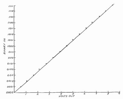
Fig. 5. Voltage output vs. binary input for Fig. 4.
