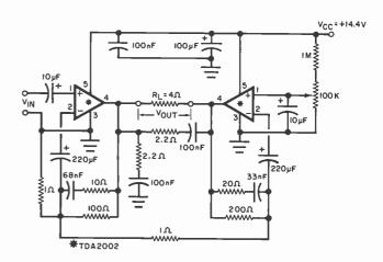
Fig. 6. Power amplifier bridge configuration.
