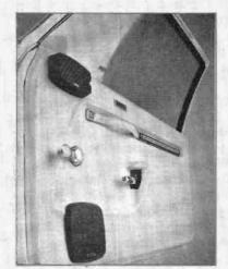
Jensen Triaxial® for front door panels has low-mounted 5¼" woofer, and surface-mounting mid-high module.
