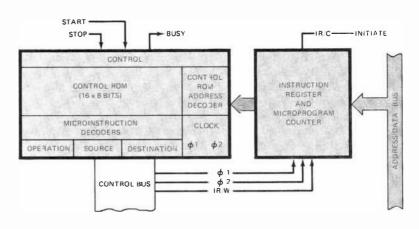
Fig. 1. Organization of the PIP-2 control section.
