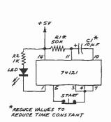
Fig. 2. A 74121 TTL monostable multivibrator.
