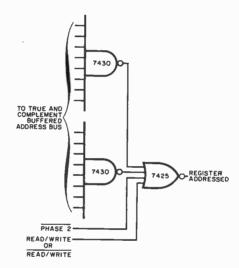
Fig. 1. Address recognizer.
