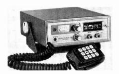
THE Model HW-2036 is the Heath Company's latest and most sophisticated vhf FM amateur transceiver. Among its features are synthesized coverage of any 2-MHz segment from 143.5 to 148.5 MHz in 5-kHz increments, true FM transmitter circuitry, dual-conversion receiver with MOSFET front end, and a 10-watt minimum-output power amplifier designed to operate into an infinite VSWR without failure.
