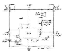
Fig. 4. Astable-monostable divider.
