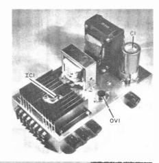
11746). Although the single-unit price is about \$14, this one device does save the several components that would be required to use a low-current regulator drive with a series-pass transistor. It is also much simpler to use.
