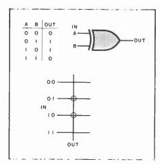
Fig. 3. At upper right is the logic symbol for Exclusive-OR, with its truth table at left.
