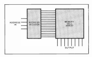
Fig. 1. How an address decoder simplifies access to a word stored in a ROM or R/WM.
