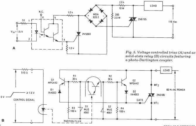
In the second circuit, Fig. 5B, the triac's ac gate signal is supplied on alternate half cycles through pnp and npn transistors Q1 and Q2 and isolation diodes D1 and D2, respectively. The transistors, in turn, are controlled by the optoelectronic coupler.
