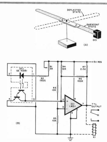
Fig. 3. Compass magnetometer's sensor (A) is a magnetic needle whose motion is sensed optically. Circuit (B) provides a TTL-compatible output and, if desired, activates a relay.
