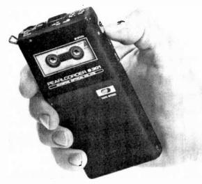
The most portable tape formats are the new "mini" and "micro" tapes, used in machines like this Olympus Pearlcorder.
