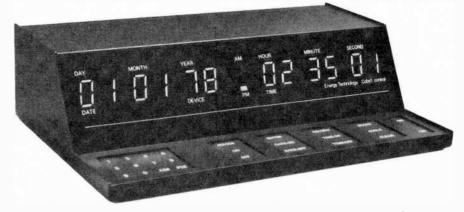
The Coby 1 Control has 24 keys to provide remote control information.
