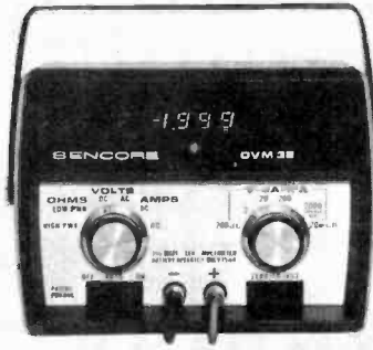
DVM32 $198 3½ digit LED display, .5% DCV accuracy, battery or AC operated with automatic battery saver
