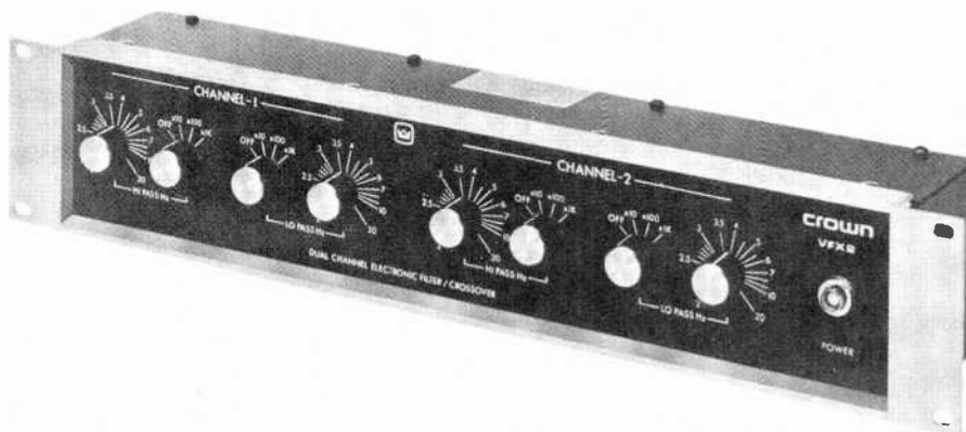
The Crown International Model VFX-2 two-channel crossover network has fixed 18-dB/octave rolloff.
