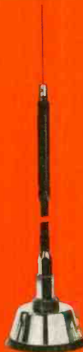
*MODEL 2-222. MOBILE ANTENNA. High efficiency fiberglass. Trunk lip mount. 50" high. Chrome plated brass cup assembly and 17-foot low loss coax cable assembly.
