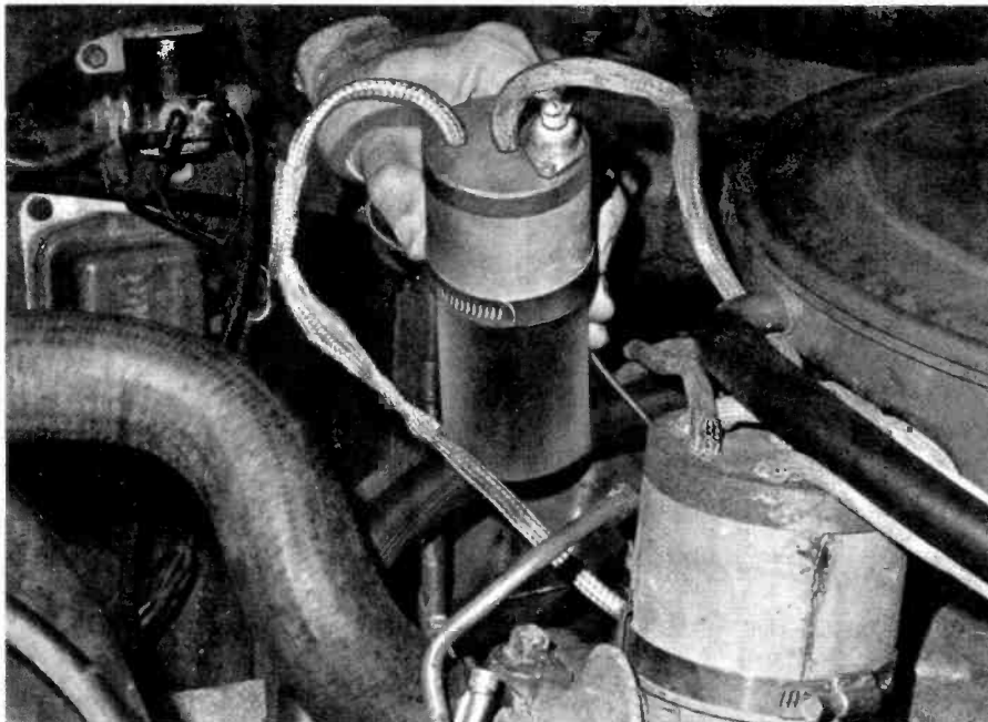
The ignition coil is shielded where the wires connect to it. Shield braids are pulled over the primary wires going to the coil.
