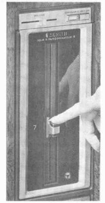
Choosing channels on Zenith's color TV receiver line is accomplished with non-detented slide control
