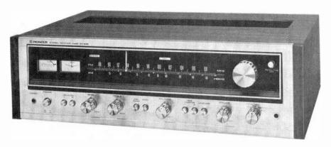
CUGHLY in the middle of the current line of stereo receivers from Pioneer, the Model SX-636 features a tuner section that makes the most effective use of integrated circuit technology that we have yet seen in a hi-fi component. The result is a level of performance, in a moderate-priced receiver, that in some respects surpasses that of most separate components—to say nothing of far more expensive receivers.
