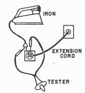
indicator. Plug an extension cord into a wall receptacle and locate the hot side of the cube tap on the end of the cord. Plug one lamp lead into this side. Now plug one prong of the cord of the device you want to test for continuity into the other, grounded, side of the cube tap. Touch the free lamp test lead to the free prong of the line cord of the device. A glow of the lamp indicates continuity.
