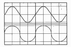
Fig. 3. Lower waveform shows effect of Dynaguard action on sine wave and lack of high-order harmonics.
