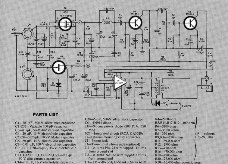
Fig. 2. Receiver employs toroid-wound coils for L1 and L2. Q1 is a dual-gate MOSFET.
