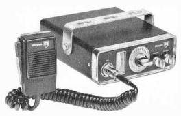
THE moderately price Model 1-600 solid-state mobile CB transceiver from Royce Electronics features crystal-synthesized operation at full legal power on all 23 AM channels. It has a meter that indicates relative signal strength on receive and relative output power on transmit. Additionally, the transceiver incorporates only the main essentials: adjustable squelch, a-f volume control, au-
