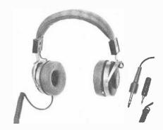
THE Pickering Model OA-3 "openair" stereo headphones provide little or no isolation from room sounds. Unlike conventional isolating-type phones that have air-tight seals betweeen the ear-cups and the listener's head, the Model OA-3
