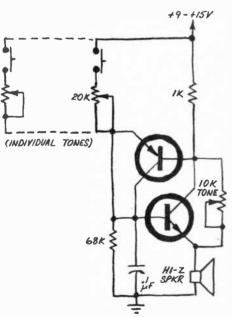
tone when a switch is closed. The one shown here uses a pair of transistors and as many switches as you wish. Each switch is associated with its own tone-control potentiometer so you can adjust each one differently. If you don't have a high-impedance speaker, try an ordinary transistor output transformer and speaker. Any generalpurpose transistors can be used.
