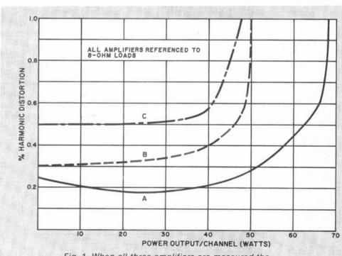
Fig. 1. When all three amplifiers are measured the same way, "lower spec" amplifier A turns out to be the highest powered unit among the three.
