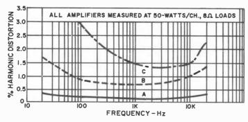
Fig. 2. Again, amplifier A proves to be much lower in distortion than amplifiers B and C, in spite of its more conservative published spec.
