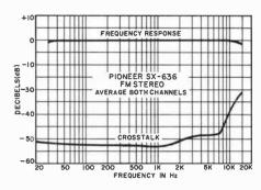
The capture ratio was an impressive 0.7 dB, about the best we have ever measured in a tuner. AM rejection was 51 dB. Image rejection was 75.5 dB, alternate-channel selectivity was 63 dB, and muting threshold was 2.2  $\mu V$ —the last low enough to exclude noise but not any receivable signals. Automatic mono/stereo switching occurred at 2.5  $\mu V$ . The 19-kHz pilot carrier leakage into the audio outputs was 41 dB below full modulation.
