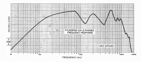
The published specifications of the Model OA-3 phones indicate that they are quite efficient, requiring only 0.1 volt across their nominal 15-ohm impedance to produce a 100-dB sound pressure level (SPL) at 1000 Hz. The maximum rated input power is 0.2 watt/channel, but the series resistors built into all amplifier headphone output circuits will provide adequate protection even with a high-powered amplifier. The distortion is specified at 0.5 percent for a 110-dB SPL output.
