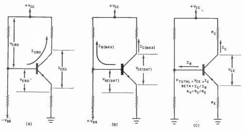
Fig. 2. Transistor is shown cut off (A), saturated (B), and in normal mode (C).
