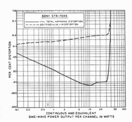
compared to other receivers in the STR-7045's price range—and even some much more expensive receivers. From a mere 0.065 percent at 0.1 watt, it fell to about 0.01 percent between 5 and 30 watts output and reached only 0.1 percent at 38 watts output.
