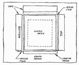
Fig. 4. Set up work area on graph paper. Tape down and identify Mylar film so that sheets open alternately to left and right.
