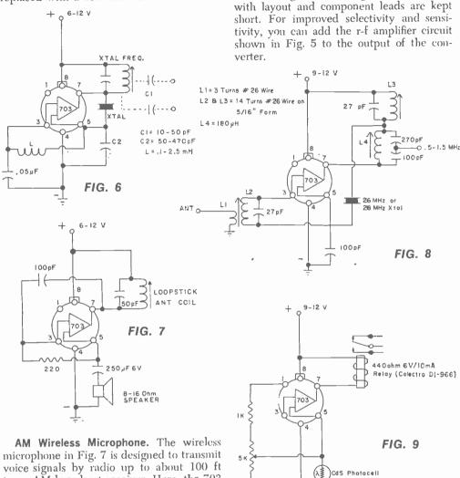
AM Wireless Microphone. The wireless microphone in Fig. 7 is designed to transmit voice signals by radio up to about 100 ft to an AM broadcast receiver. Here, the 703 IC is used as an oscillator and audio amplifier. Only a small transistor radio speaker is needed as a microphone. For use as a phono-oscillator, replace the speaker with a 50,000:1000-ohm transformer, and connect the high-impedance winding to the phono cartridge.
