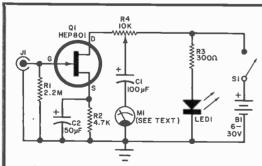
Simple VU meter uses FET input stage for high impedance and amplification to drive meter (with diode bridge).
