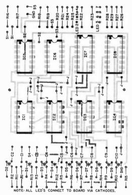
Fig. 3. Indicate exact location and orientation of each component on layout diagram.
