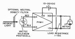
Fig. 5. Photocell voltage multiplier (Model PVM-1 by Vactec) increases the sensitivity of the selenium photovoltaic cell at left.
