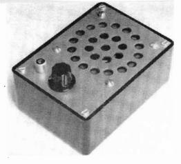
Front of receiver has holes drilled for antenna jack, speaker, and sensitivity control.
