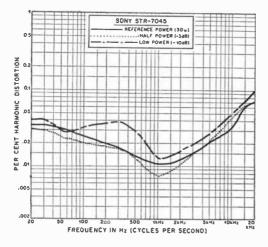
Sony's conservative power ratings were emphasized by the fact that at the rated 30 watts/channel (or less), the THD was under 0.1 percent at any frequency from 20 to 20,000 Hz and was typically about 0.02 percent.
