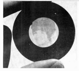
Fig. 7. Photographic image stored in Sandia Cerampic is ready for projection like slide.
