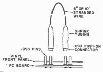
Fig. 3. How to make interconnecting jumpers. Make up about 24 of them.
