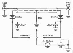
with a 4½" piece of RC-58A/U coaxial cable and a similar length of ¼" copper tubing. Remove the outer jacket and braid from the coax, leaving only the insulation and the inside lead. Locate the center of the cable and gently cut away the insulation so that a 51-ohm, ½-watt resistor can be soldered to the center conductor—but don't solder it on yet.
