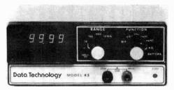
power supply and amplifier circuits. It has five ac and dc voltage ranges with  $10\text{-}\mu\text{V}$  resolution, six resistance ranges with 10-milli-ohm resolution, and five each direct and alternating current ranges with 10-nA resolution. The instrument will operate for 10 to 12 hours on fully charged batteries. Power consumption is 3 watts, and the 7-segment display measures 0.33'' high. The calibration chart is silk-screened inside the case so that it cannot be mislaid. Price is \$399.
