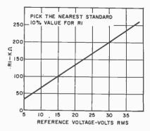
Fig. 3. Use this chart to deternine value of RI (Fig. 2) when 60-Hz reference voltage level in rms is known.
