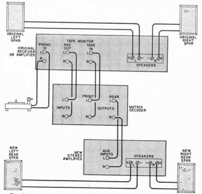
Fig. 2. First-generation quadraphonic hookups used separate decoder connected to the tape monitor jacks of the existing stereo system.
