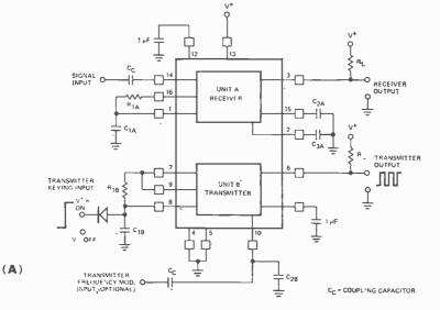
Fig. 2. Two applications for the XR-2567 dual tone decoder. In the duplex tone transceiver circuit shown at (A), unit A serves as a tone receiver and unit B as a tone transmitter. In (B), at right, only half of the IC is utilized to form a precision oscillator of ruse in circuits such as a musical instrument tone generator.
