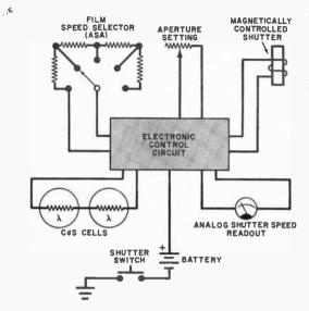
Fig. 3. The simplified electronic interconnections for aperture priority system such as that used in the Pentax ES. The ASA selector and aperture setting both program the camera. The electronics then takes that information plus the stored light meter reading from photocells and calculates the proper amount of time to keep the shutter open for correct exposure. The shutter speed is read out for various apertures (f-stops) on the meter which is seen through the view-finder.
