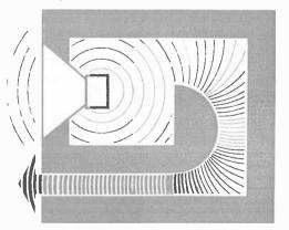
Cavity behind BIC venturi's woofer tapers into duct that opens into listening room.
