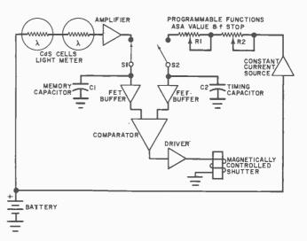
Fig. 2. The principal components that are employed in an electronic exposure system. Voltage on CI depends on the lighting that is on subject.
