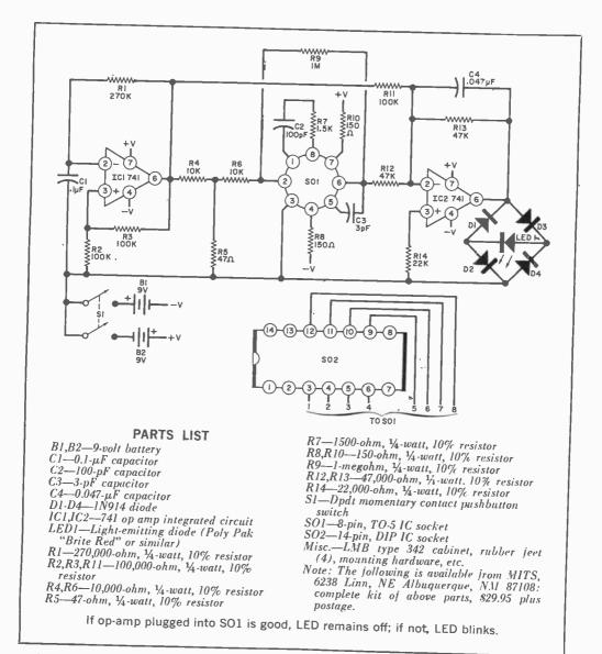
with the two batteries. The LED was glued (with epoxy) to protrude through a small hole in the front of the cabinet with SI mounted beside it. Four rubber feet on the bottom of the cabinet will keep the tester from slipping around when in use.
