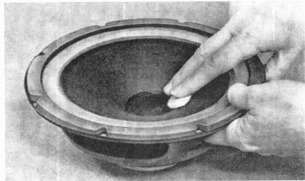
Modeling clay is pressed against the speaker cone to change mass of speaker.
