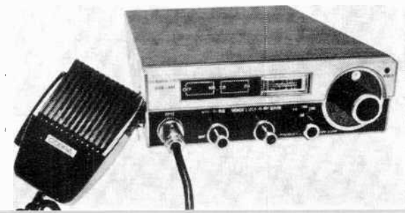
Dynascan "Cobia 132" is a compact single-sideband/AM mobile CB rig.
