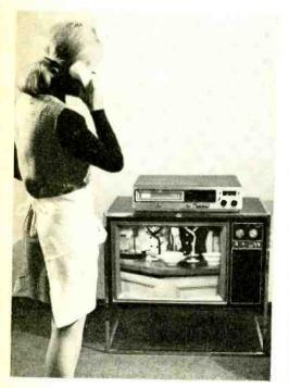
ridge. A set of piano key switches are used to control the various operations. The only connection between the player/recorder and the TV set is through the antenna terminals. The set is tuned to an unused channel for tape operation.
