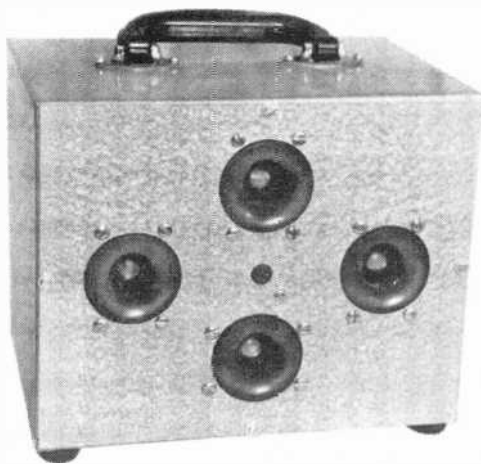
Arrange drivers as shown for best dispersion and maximum acoustical output.
