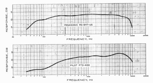
program advance and four lights which indicate the channel and mode in use. Its 125-mV output and -37-dB noise levels were close to the group average. The uniform frequency response over most of the
