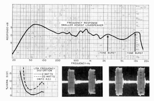
At top is shown frequency response curve and points at which tone burst tests were made. Photos of tone burst reproduced are shown above right. Above left is graph of low-frequency distortion of the speaker at 2- and 20-watt levels.
