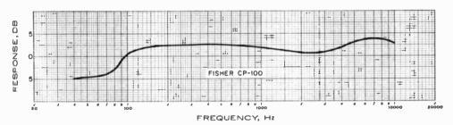
• Fisher CP-100 (\$169.95), In its measured performance, Fisher's CP-100 was typical of the test group, its output—not necessarily the maximum or minimal level—was 120 mV from the reference 1000-Hz tone on the tape. Noise level was -38 dB relative to the 120-mV level.
