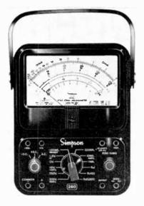
function switch set to TRANSIT, the meter's pointer movement is damped during its travel, thus preventing G forces from bending the pointer.
