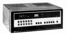
a master board. Tuning frequency, derived from a digital frequency synthesizer employing phase-locked loop techniques to achieve tuning accuracies of better than 0.005%, is displayed on four 7-segment Numitrons. Tuning is accomplished by punching in the frequency of the station desired via a 10-button panel; by operating a sweep/scan switch; or by using any one of three buttons for activating the appropriate builder-punched computer memory card.
