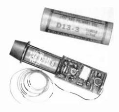
RECENTLY, we had the opportunity to build and test the "Transroc" model aircraft and rocket transmitter put out by Estes Industries. Since it was designed to be used in conjunction with a conventional Citizens Band receiver, we were surprised at the compact size of the six-transister, crystal-controlled transmitter.
