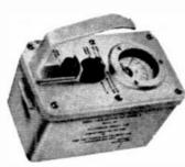
You can buy a complete radiation meter, complete with original instruction books, at less than the price of the meter movement a lone. Range is 0.02 to 50 Roentgens/ hour. This is not sensitive enough for nrospecting but usefulforother radiation measuring and monitoring purpases. If not used for its original function, then the case,
