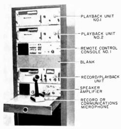
Fig. 3. Front view of control console.
