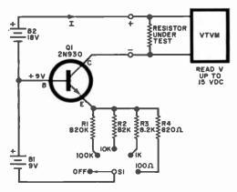
Test resistance value is equal to voltage drop across resistor times range multiplier of current source.
