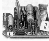
Encapsulated video color driver requires no heat sink for transistors.
