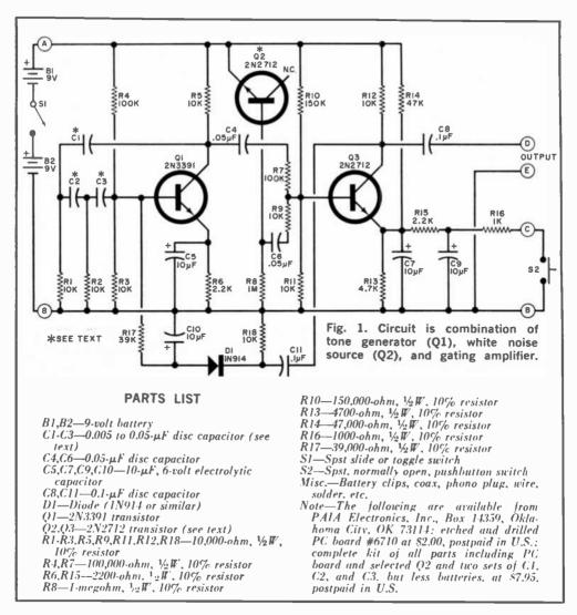
Note how components are connected to board with S1 between the batteries.
