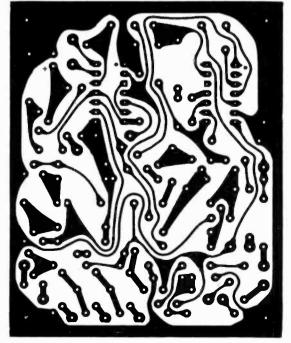
Fig. 5. Actual size drilling and etching guide and component placement and orientation diagram are shown left and below, respectively.
