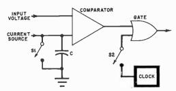
Fig. 1. Elementary capacitor-discharge analog-to-digital converter is typical of those used in digital instruments.
