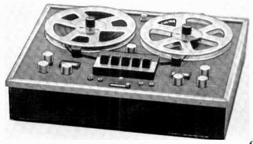
frequency response to beyond 12,000 Hz, which is adequate for taping almost all disc records and FM broadcasts. These two speeds are offered on virtually all home tape recorders, frequently in conjunction with a 1%-ips speed. Vocal material and background music can be recorded with adequate fidelity at 1% ips, but the upper frequency limit is usually between 6000 Hz and 10,000 Hz.
