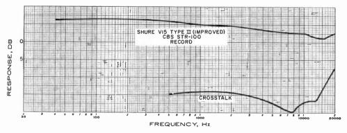
Frequency response and crosstalk curves for Shure V15 Type II (Improved) phono cartridge were obtained using CBS STR-100 record.
