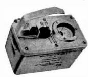
You can buy a complete radiation meter, complete with original instruction books, at less than the price of the meter movement a lone. Range is 0.02 to 50 Roentgens/ hour. This is not sensitive enough for prospecting, but useful for other radiation measuring and monitoring purposes. If not used for its original function, then the case,
