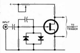
Input sensitivity is controlled automatically by this circuit in Weston counter.
