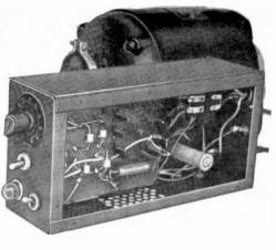
loads. The full-wave circuit provides speed control, reversing, and dynamic braking.
