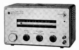
output impedance on all functions and ranges is less than 3000 ohms.
