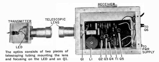
gree of selectivity. The rest of the amplifier is conventional transistor stages itilizing relatively large resistance values to minimize dc current drain. Because the IR beam is chopped, it is possible to use ac-coupled amplifiers which are easily built to operate at low power.
