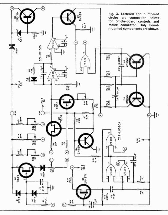
plied to the integrator resistors. R5 and R6 through ZERO set control R2 and D3. Transistors Q2 and Q3 act as switches for the integrator and reference currents.
