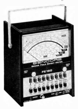
size is to permit the front panel to accommodate comfortably 18 pushbutton switches which replace the traditional rotary range and function switches found in most multimeters. These switches can be used in the proper combinations to provide up to 112 measurement ranges!
