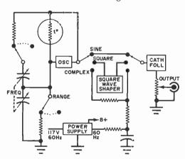
Feedback thermistor maintains good amplitude stability and reduces distortion.
