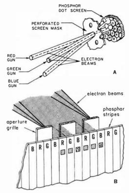
Fig. 2. At top is shadowmask scheme; below, Trinitron CRT aperture grille.
