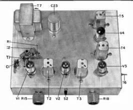
Fig. 2. This view of the top of the tuner shows how components were arranged on chassis for the prototype.
