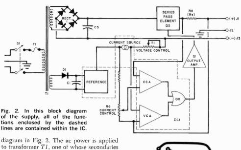
diagram in Fig. 2. The ac power is applied to transformer T1, one of whose secondaries supplies bridge rectifier RECT1 and filter C3 to provide unregulated dc for the overall regulator. The other secondary supplies rectifier D1 and filter C1 to create the dc power required by the reference voltage regulator in IC1.
