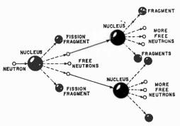
Nuclear fission occurs when a highspeed neutron splits nucleus of uranium or plutonium. Tremendous energy is released and other neutrons are knocked loose. If released energy is sufficient, chain reaction can occur.
