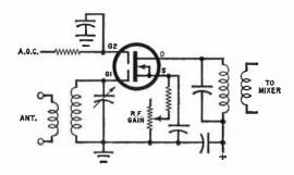
Fig. 3. Here, the dual-gate MOSFET r-f stage has its gain controlled by a negative voltage which shown is applied to gate 2.
