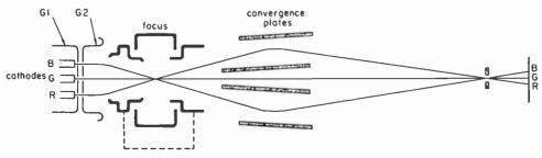
the same ones that let two green beamsegments through—pass only enough red beam to illuminate two red stripes of phosphor. The angle of the red beam just suits the positioning of the red stripes with respect to the grille openings, and the red beam does not touch green or blue stripes.
