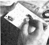
Assembling integrated circuit on a printed circuit board — Circuit is identical to one used in latest IBM System 360 computers. Student is constructing an oscillator combined with a Darlington pair output amplifier.
