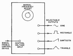
In audio tone oscillator, frequency of the output is adjusted by control knob or by use of an external signal.
