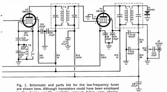
Fig. 1. Schematic and parts list for the low-frequency tuner are shown here. Although transistors could have been employed in the design, readily available vacuum tubes were chosen. Note that two r-f stages (V1 and V2) were used in design because the low power of the transmitter requires a very sensitive tuner. The converter stage is V3, and V4 is the amplifier.
