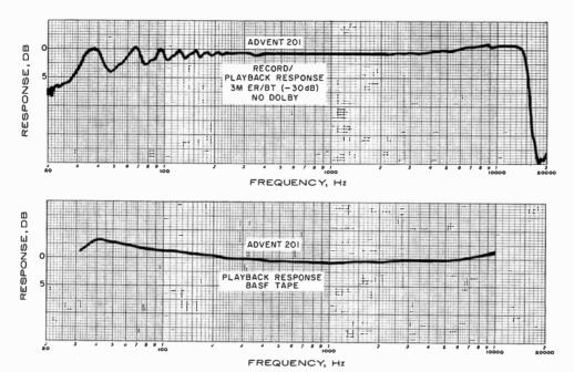
Record/playback (top) and playback only (directly above) curves show the Advent 201 tape deck's very flat frequency response over range of 50-10,000 Hz.
