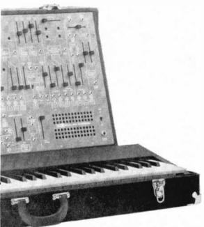
Portable synthesizer made by ARP Instruments (Div. of Tonus Inc.)
