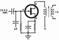
Fig. 5. This circuit shows how a junction FET can be used as mixer. There is less isolation than when the dual-gate MOSFET is employed.
