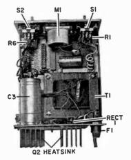
This shows the completed supply except that the small board is not plugged into the edge connector so that it doesn't hide other parts.
