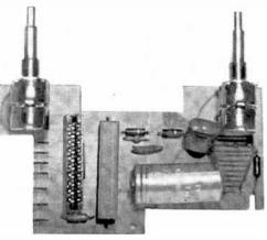
Fig. 5. Completed boards should look like these. The two dual potentiometers mount big board to chassis front.
