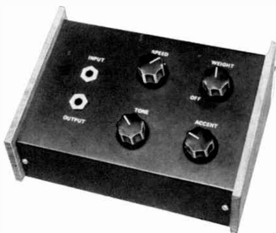
In prototype, top of case slopes downward. Top, front, and rear panels are painted flat black to contrast with rich tones of walnut side panels. Controls and jacks are lettered in white, using dry-transfer lettering kit.
