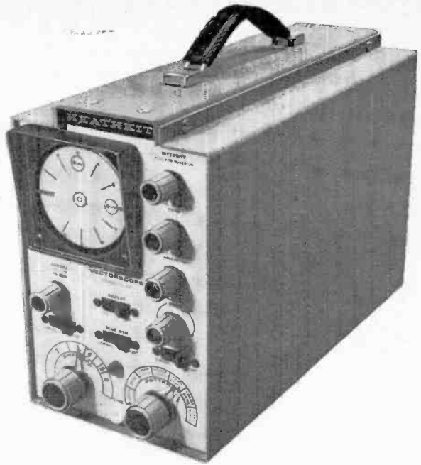
The Heathkit IO-101 Vectorscope is a lightweight self-contained test instrument for setting up convergence, purity, and gray scale of any color TV receiver. Much of the wiring (to left) is on a printed circuit board and relatively easy to handle. Rear of the instrument has hooks for retaining necessary interconnecting cables to color TV receiver. Note "chroma" switch which permits use of Vectorscope with any picture tube feed circuit arrangement.
