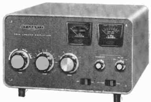
Top-value linear amplifier is this new item from Heathkit—Model SB-220. With a 2-kW p.e.p. SSB and 1-kW CW/RTTY rating, it sells for about $350. The SB-220 also has A.L.C. and a drive requirement of 100 watts for full rated input/output.
