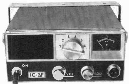
Solid-state Varitronics/Inoue IC-2F has a FET front end and IC's in the audio if stages. The output is 10 watts of crystal-controlled narrow-band FM.
