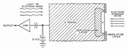
Fig. 1. Silicon Intensifier Tube (shown in blocked portion of diagram) incorporates special light amplifier and a silicon integrated circuit as its retina.
