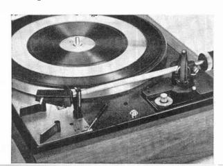
Special features of Dual 1219 include disc diameter selector and damped up/down cueing levers (far left foreground) and antiskate and tonearm leveler controls (near left foreground). Cast platter is a full 12" in diameter and comes with mclded neoprene ribbed disc mat.
