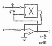
Fig. 4. Motorola IC operates in all four quadrants; puts low-cost calculator in reach of experimenter.
