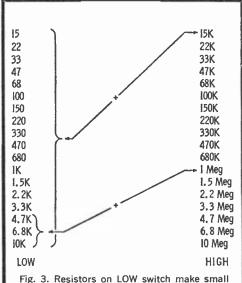
Fig. 3. Resistors on LOW switch make small changes in total resistance selected by HIGH switch. Illustrated are combinations of settings between 15,000 ohms and 1 meg.
