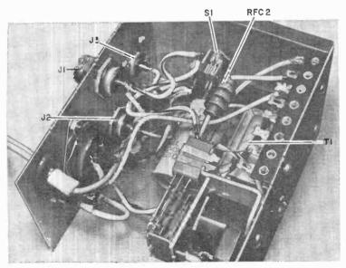
The current threshold detector circuit made up of D1, D2, and T1 controls the power delivered to the solenoid of K1. The voltage drop across monitoring diodes D1 and D2 is on the order of 1.5 volts peak-to-peak and is independent of the power required by the transceiver. The square-wave voltage drop across the diode pair is coupled through transformer T1 to silicon controlled rectifier SCR1.
