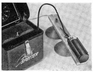
Transducer slides into strong, boardmounted retainer. Large suction cups on board permit attachment to nonporous hull of boat, while nylon safety line prevents assembly from tearing away in event suction cups work loose.
