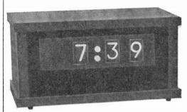
counter chain which uses the 60-Hz line as a reference with decimal and divide-by-six counters feeding BCD-to-decimal decoders. If I were to build another one right now, I could do it for a little under \$90.
