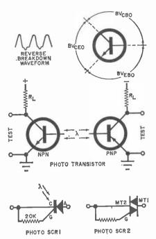
Fig. 3. Reverse breakdown of transistors can be determined, as well as the operation of several types of light-sensitive semiconductors. The two circuits at the bottom show how to wire these semiconductors.
