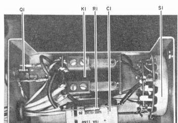
Fig. 2. After mounting components in small utility box or under dashboard, try to water-proof circuit to prevent relay and switch contact corrosion.
