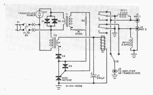
Fig. 1. Lightning protector features switching facilities for two antennas. Use fused plug for supplying power to obtain maximum lightning protection.
