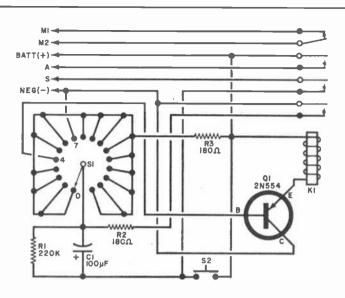
Fig. 1. Combination sequence is 7-4. Simple rewiring of S1 allows selection of any other two-digit combination desired.
