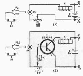
Fig. 1. Circuit in (A) is used for short runs where line voltage drop is minimal; (B) circuit provides current gain through Q1 for long runs.
