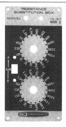
Fig. 5. After making modifications, front panel of substitution box must be reworked to indicate new switch position markings.
