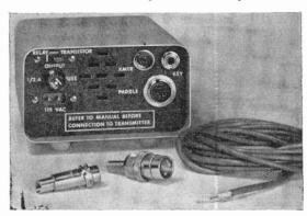
Rear apron of Curtis EK-38 electronic keyer accommodates all external cable connectors, a relay/transistor output selector switch, and power fuse. Mating connectors and cables (shown in foreground) are supplied with kit.
