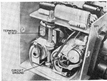
grounds should be made to the same grounded battery clip where the negative end of C15 is connected.
