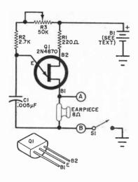
Fig. 1. Simple UJT relaxation oscillator makes up repeller; output is from earpiece.
