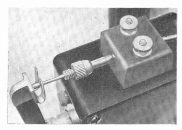
cate and drill the exit hole for the arm of the solenoid, centering it between the two sides of the box. Then drill the mounting holes for the solenoid and actuating arm pivot bracket, and for the potentiometer (located directly opposite the exit hole for the solenoid).
