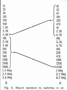
Fig. 4. Mount resistors to switches in order shown here. Each switch should contain half of the resistors less than and half greater than 10,000 ohms when you finish.
