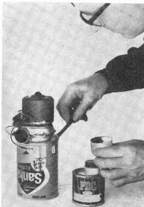
Fig. 2. The small fan is cemented to its hole in top of can. Make sure that the joint is airtight.
