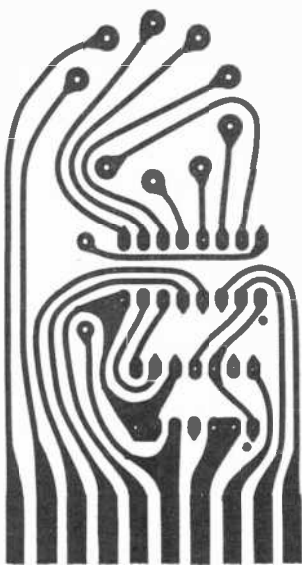
Fig. 2. Actual size printed circuit foil pattern for the readout.
