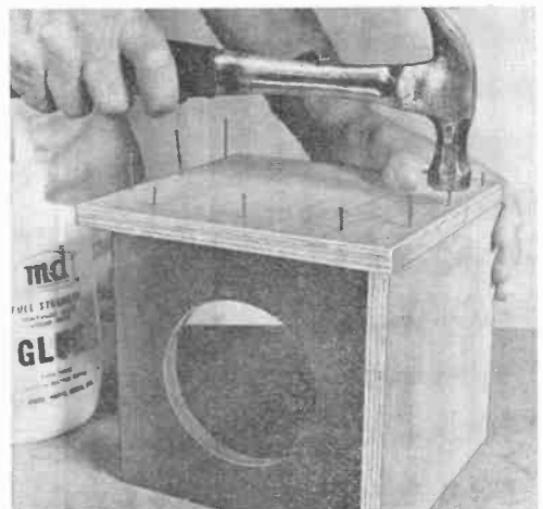
Fig. 3. Before assembly, start finishing nails into top, bottom, and rear walls of cabinet. Then apply beads of glue and hammer home nails as shown here.
