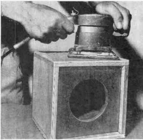
Fig. 6. Power sander is fast way of smoothing surfaces, but you can use wood block and sandpaper.
