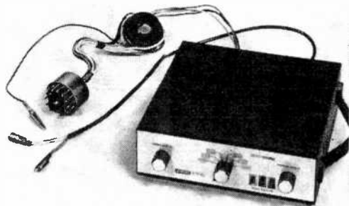
In the view of the Color Bar chassis, above right, the printed circuit selector switch is at the top of the photo while battery clamps on back of chassis are at bottom.
