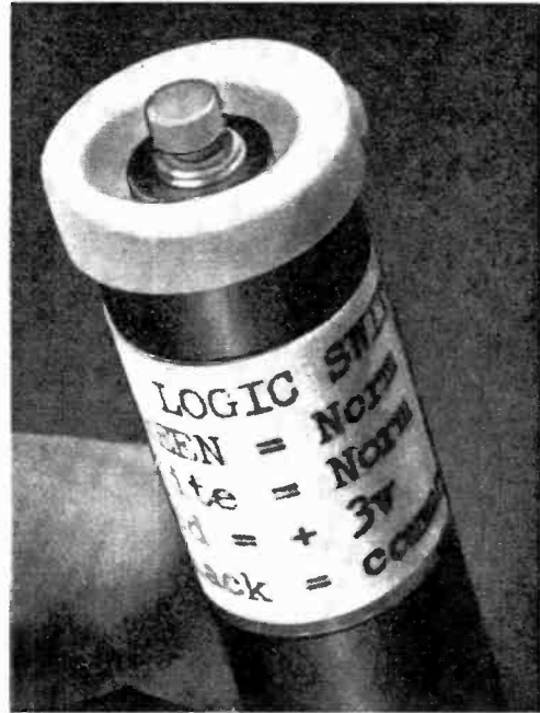
The pushbutton switch fits in a hole drilled in container cover. Like other testers, a typewritten label identifies leads and explains operation.
