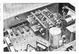
Ultra-Monitor has unique functional design and is very light weight. Oval speaker is mounted behind grill under the carrying handle. Receiver contains rechargeable batteries. Pilot lights on front panel indicate whether or not batteries are being recharged and if Tone Alert has been activated.
