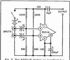
Fig. 2. The KD2116 makes an excellent twochannel mixer useful for audio systems.
