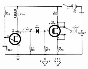
Fig. 3. With the addition of a MOSFET, only positive-going pulses from Q1 are used. Phase splitting then provides a repetition rate of 400 pps of either polarity.
