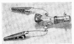
A broadcast-band filter is used with the marine-band converter to eliminate pickup from strong broadcast stations that might cause undesired breakthrough.
