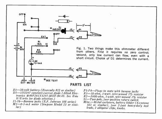
tions to S1, be sure that the correct terminals are used on each section. Also be sure that D1 is wired in correctly. If you use the Motorola diode called for in the parts list, the black band should be to-
