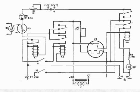
Fig. 1. Once system is tripped, relay operation is in numerical sequence. As K2 closes, it pulses shutter solenoid; K2 provides the power-disconnect feature.
