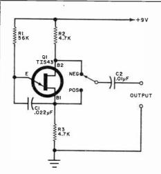
Fig. 1. Simple unijunction transistor circuit generates positive or negative pulses of relatively wide durations.
