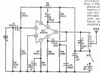
Fig. 6. An excellent wireless microphone can be made using the KD2114. Speech quality is very good (with the microphone suggested), and range is about 50 to 150 feet, depending on receiver used and its antenna.
