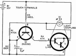
Fig. 3. Touch control circuit uses photo-Darlington transistor, which, once triggered, is held on by 11.
