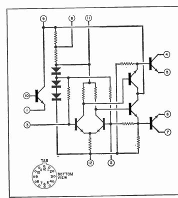
Fig. 3. The KD2115 is complete audio amplifier in a TO-5 can. When driven from a low-level signal, this IC can put about ½ watt to a speaker. Because of its low power requirements, and small size, it makes a good general-utility bench amplifier, as well as a handy amplifier for outdoor (battery) operation.
