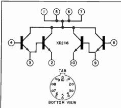
Fig. 1. The KD2116 consists of four closely matched npn transistors arranged in a pair of Darlingtons. All collectors are common.
