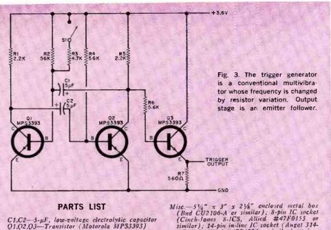
C1,C2—5-µF, low-voltage electrolytic capacitor O1,O2,O3—Transistor (Motorola MPS3393)
