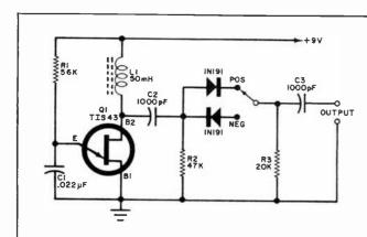
Fig. 2. This circuit generates positive and negative pulses simultaneously with the shape of the pulse sharpened by the inductor in the base 2 circuit.
