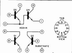
Fig. 5. The KD2114 also contains four npn transistors, arranged as an isolated pair and a Darlington. Each transistor of the Darlington can be used independently when certain external circuit changes are made.
