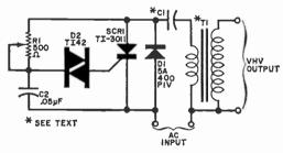
By driving the very-high-voltage power supply with a variable-voltage transformer, output voltage can be made to vary above and below 10,000 volts.
