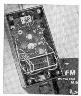
Completed, mounted wireless microphone fits into small plastic case. Tuning capacitor C7 is accessible through a small hole in the plastic cover.
