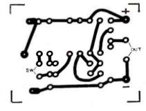
Fig. 4. Actual-size foil pattern for the oscillator.
