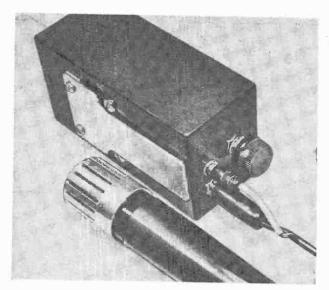
A metal strap arrangement can be mounted on the rear of the plastic case so that the wireless microphone can be carried on the user's belt. The microphone can be hand carried or mounted on a neck strap for lavelier mike.
