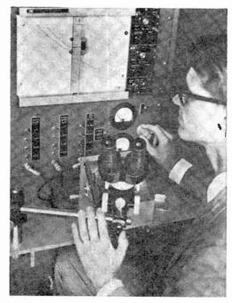
Fig. 1. Inventor John A. Copeland, Bell Telephone Laboratories, uses new Profilometer to plot the densities of impurities in a semiconductor wafer.
