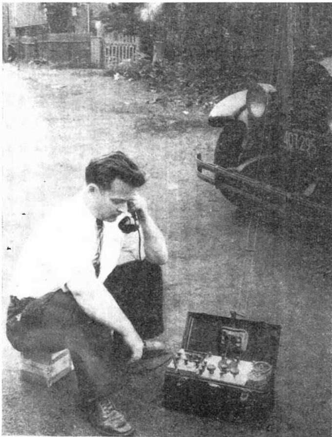
This is what a portable transceiver looked like in 1933. The antenna was mounted on a wooden pole supported by the car radiator—not exactly a mobile installation. (Photo: National Radio Company, Inc.)
