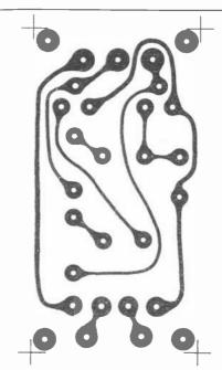
Fig. 2. You can make an actual-size PC foil pattern by following this layout.
