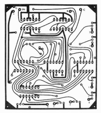
Fig. 3. Actual-size printed circuit foil pattern for the DCU. The use of this pattern is suggested because of the complexity of the circuit. Point-to-point wiring is not to be recommended.
