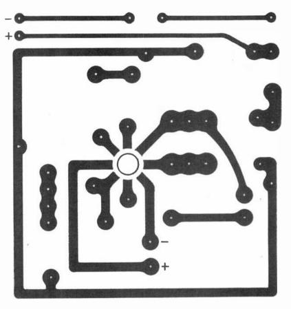
Fig. 2. Actual-size printed board foil layout. You can create this circuit on perf board if desired.
