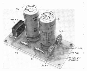
Physical arrangement of a finished PC board. Note that both capacitors are vertical to the board while other components are conventionally installed. Two connections to S1 are hidden behind the capacitors. When installing, remember that the circuit is "hot" to ground and you can get shocked if not careful.
