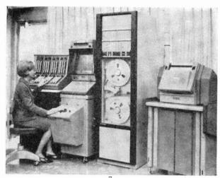
In this fax system, documents retrieved from a microfilm storage are scanned and recorded at high speed for later transmission at low speed on telephone lines. (Photo courtesy of Alden E. & I. R. Co.)
