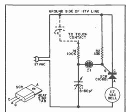
The capacitance of the body, Cx, when contact is made with lead to R1, causes voltage on C1 to break down I1 and fire SCR.
