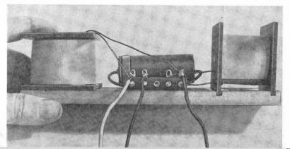
wire out through the remaining holes in the coil forms. Scrape away about ½" of the insulating enamel from the free ends of the coil windings.
