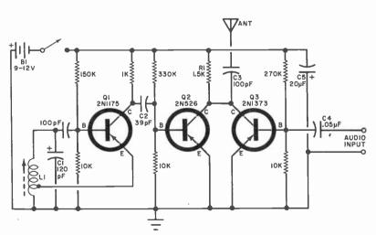
Fig. 3. Unusual AM transmitter circuit has modulated buffer amplifier to improve overall stability of audio system.
