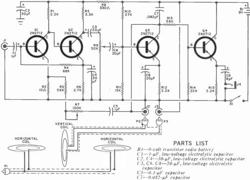
Fig. 1. Basically an unstable high-gain audio amplifier, the circuit breaks into oscillation when metal is detected between horizontal and vertical coils.
