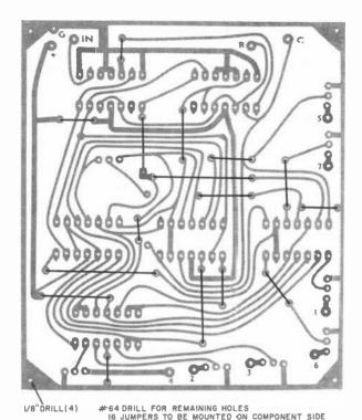
Fig. 4. Other than the four corner holes (for mounting), use a #64 drill for all holes, Wire the required 16 jumpers on the component side of the PC board.
