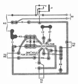
Fig. 3. Install the components as shown here. Note that J1 is arranged to close when plug is inserted.
