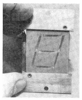
Fig. 1. Front view of the commercial seven-segment readout showing the numerical pattern. Mounting frames are available to hold several such readouts.
