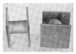
Fig. 3. Each Masonite section is  $2\frac{1}{4}$ " square by  $\frac{1}{8}$ " thick; wood dowel is  $1\frac{7}{8}$ " long by 1" diameter.
