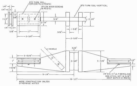
Fig. 2. Except for copper wire in the three coils, no metal is used in the search head construction. Nylon screws secure the two horizontal coils. Use a strong glue or cement for overall assembly.
