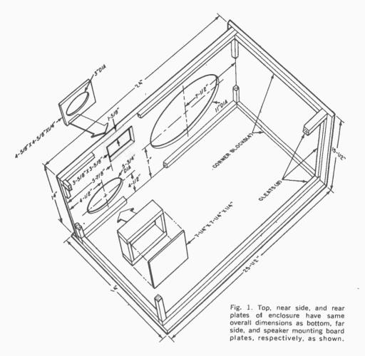
in Fig. 1, prepare the main enclosure's rear plate, speaker mounting board, and cleats and corner blocks. (Note: Only one side, the bottom, and the speaker mounting board are illustrated in the drawing. The remaining side is the same size as the side shown; the same applies to the rear and top plates, which are identical in size to the speaker mounting board and bottom plate respectively.)
