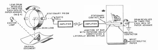
Electromechanical scheme of a typical 96 line/inch "message fax" system which records document in slotfed scanner at left and reproduces it on recorder at right. Roll feeding of recorder is now common method.
