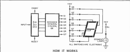
The heart of the third-generation counter is a single-plane, seven-segment display in which individual segments remain stationary and are illuminated in various combinations to produce the necessary numeral.
