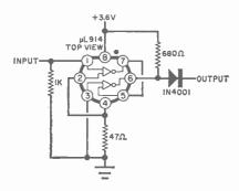
Fig. 9. This shaper will convert a sinewave to a square wave of same frequency.
