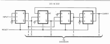
Fig. 2. The logic circuit (above) accepts the input pulses and produces certain discrete voltage levels at the outputs. The decoder (right) processes these voltages and causes only certain matrix segments to remain lit, creating a number.
