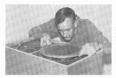
Fig. 2. To insure proper air seal, be sure to place rubber, felt, or other adequate gasker material between speaker rims and speaker mounting board.
