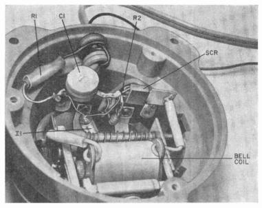
The entire circuit is easily accommodated in bell housing. Be sure that there are no short circuits when the cover is put back on the bell.
