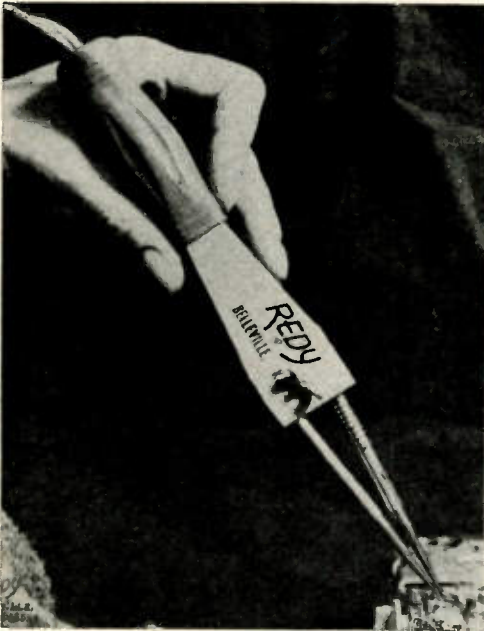
This is a tweezers-type electrode assembly that is commonly used with resistance soldering equipment.
