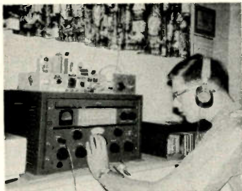
Mike Wright, WA7HRE, Scottsdale, Ariz., worked 48 states and 21 countries as a Novice using a homebrew 70 watt'er, a Collins 75A-1 receiver—a gift from his father, W7IMA—a 2-element, 15-meter beam, and a 30-foot vertical to work the 40-meter band.
