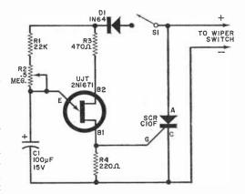
Fig. 1. The SCR supplies power to windshield wiper motor in this slow-kick control for so-so weather.
