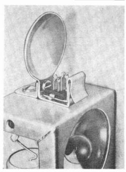
The "hot" lead to the AG-1 flashbulb socket is passed through a hole in the top of the chassis. The other connection is made through the spring clip.
