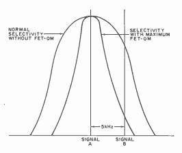
Fig. 2. Broadcast signals 5 kHz apart can be easily separated with the FET-QM in the receiver's circuit; unwanted signal B is greatly attenuated.
