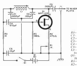
Fig. 1. High-Q 455-kHz tuned circuit (C1, C2 and L1) helps narrow passband of receiver, while R1 in source of Q1 provides means for controlling regeneration.
