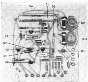
+6VDC Fig. 5. This Gate mod-II OVERRANGE ule circuit is the basic timer for the DVM. QI MPS 2923 Q2 MPS2923 Q3 MPS2923 QI-Q3 R5 470Ω § C4 /.DOIµF IC4 µL900 +3.6VDC R3 3.3K IC3 µL914 ICI MC789P IC2 MC790P в\* 4 ₹ RI 220K
