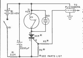
Fig. 1. The circuit will not operate until the gate of the SCR is triggered by a pulse from the camera's internal flash battery.
