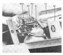
The bulk of the components are wired point-to-point on the terminal strip. The coaxial cable to the camera enters the chassis via a small rubber grommet.
