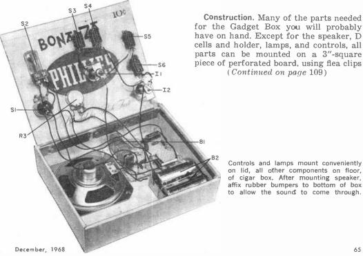
for the Gadget Box you will probably have on hand. Except for the speaker, D cells and holder, lamps, and controls, all parts can be mounted on a 3"-square piece of perforated board, using flea clips (Continued on page 109)
