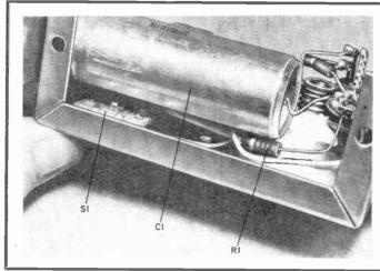
Storage capacitor C1 extends the length of the small chassis. One end is tied to the terminal strip; the other end is connected to the common ground (chassis) via a small soldering lug. Resistor R1 is connected between the terminal strip and power switch S1.
