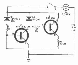
Fig. 2. If the supply increases beyond the zener diode rating, transistors saturate to light II.
