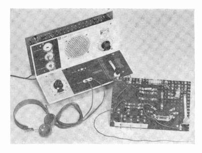
Shown here with Knight-Kit "Electronic Science Lab" (left) is the Lafayette Radio Electronics "Transistor Experimenters Kit"—the only kit requiring soldering equipment.
