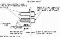
Fig. 12. Arrange lamp mounting holes in two closely spaced, staggered columns to obtain small size.
