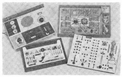
Most of the projects in the instruction manual are radio receivers or radio-oriented circuits. Projects are set up with the aid of a plastic frame and individual component cubes. All cubes (except one large block containing a tuning capacitor and loopstick antenna) measure %" on a side. Component symbols and number
