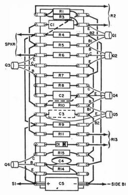
Fig. 3. Route capaciter C3 and wiring indicated by dashed lines along the underside of the tag strip.
