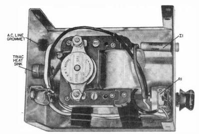
Fig. 3. When testing the magnetic stirrer with the top of, be sure not to touch any of the wiring since all of the circuit is connected to the a.c. power line. Do not use the metal chassis as a common tie point for any of the circuit.
