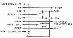
Fig. 6. Prior to wiring them into chassis, test individual DCU's using this circuit.
