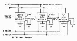
Fig. 7. Carry output of each module provides input for following module. As many modules as desired can be used; units, tens, hundreds, etc., modules.
