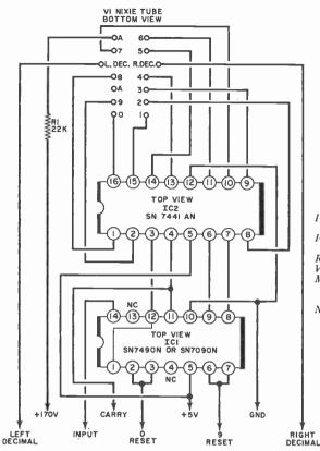
Fig. 1. Entire counting circuit is made up of four components—demodulator IC1, driver IC2, glow-discharge tube V1, and current-limiting resistor R1. Value used for R1 is determined by number of counting units operated from a given power supply, as described in text.
