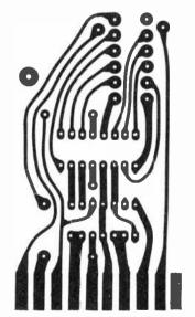
Fig. 2. This actual-size etching guide is used for circuit board employing edge connector (heavy mark at lower right serves as connector key), or for circuit board to be soldered into circuit.
