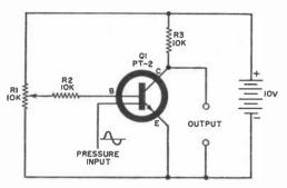
Fig. 3. The Pitran is a pressure-sensitive transducer which can be used in a standard transistor audio-amplifier circuit for various applications.
