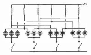
Fig. 16. In this sequencing circuit, when only one switch is closed, three lamps associated with it are lit. Subsequent closing of another switch lights only two of its lamps due to lowered voltage drop across one resistor. Last switch lights no lamps.
