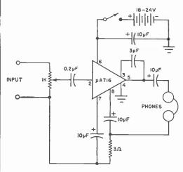
Fig. 5. Integrated-circuit headphone amplifier has good match to 600-ohm headset for high efficiency.
