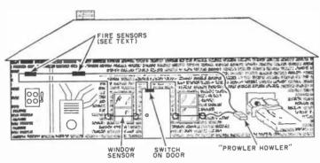
Fig. 3. Suggested layout for house intruder and fire protection. Almost any method of sensing will suffice as long as you remember that the system operates when any part of the closed loop is opened.
