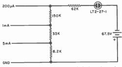
Fig. 18. To check a.c.-operated devices for safety where leakage currents are concerned, this simple circuit uses one neon lamp in series with a 67.5-volt battery. Three separate probes are used. If lamp lights when the 5-mA probe is used, leakage is too high and device is considered unacceptable.
