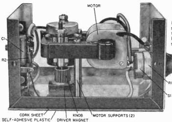
Fig. 2. View of inverted chassis shows driver magnet fixed to knob secured to motor shaft. Magnet must be as close as possible to non-magnetic frame top.
