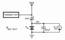
cause it also tells what the antenna is doing, the circuit shown above can be wired into your rig. The diode, D1, can be almost any signal diode you have at hand.
