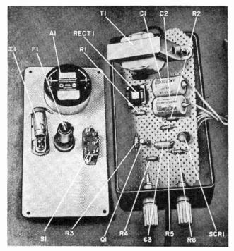
Fig. 2. The Prowler Howler is built in a 3"  $\times$  6"  $\times$  2" plastic case as shown here. If you elect to use battery only operation, the space now occupied by the a.c. power supply components can be used to mount a conventional 9-volt radio battery.
