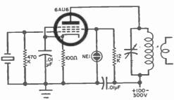
Fig. 12. In a crystal oscillator circuit such as this, the constant maintaining voltage of the neon lamp is used to regulate the screen voltage on the 6AU6, thus providing improved frequency stability.
