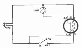
With S1 at OFF, lamp and K1 receive power until thermal action opens relay's bimetallic contacts.
