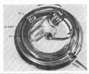
Thermal relay and switch can be conveniently mounted inside hollow base of most lamps. Glue sheet asbestos and layer of felt over base to conceal tube and a.c. line cord.
