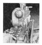
bracket provides belt adjustment. Overcharging is prevented by the car's voltage regulator. When not in use, the fan belt goes back in place and the mower engine stores neatly away in your car's trunk.
