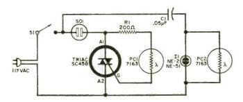
Fig. 1. Automatic light-switch circuit uses medium-power triac and light-sensitive controls to handle loads to 1000 watts.
