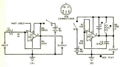
Fig. 2. Integratedcircuit square-wave converter (left) and audio oscillator can be built for auxiliary testing use in the home workshop.
