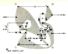
Fig. 7. Component installation on the power supply PC board. Note that R1 is two resistors in series.
