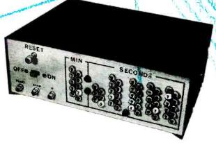
THE AVAILABILITY OF LOW-COST decimal-readout counting units has created an entirely new "ball park" of experimentation for the advanced electronics hobbyist. This new area is digital-readout instruments and we will be publishing several articles on such projects in the months to come. The first is the "Sports Timer," a real-time clock, described here.
