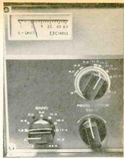
Controls on SW-4A are few and far between. Eleven tuning ranges are identified by clots and bars in various colors. The SW-4A was the only one of group with a tone control.
