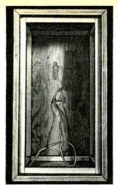
Fig. 3. Two screws, inserted through rear of enclosure, serve as electrical connections.
