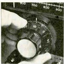
Two-speed dial knob is featured in brand-new Galaxy R-530. Skirt of knob reads in one kilohertz increments. Hairline may be shifted back and forth for adjusting dial calibration. The slide-rule dial above reads 0-500 or 500-1000.
