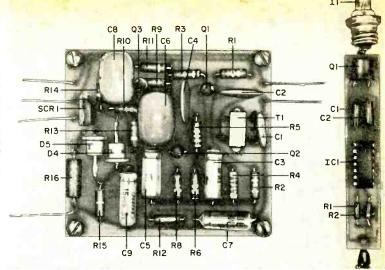
prefer to run a piece of #16 wire from the circle marked "case" on the printed circuit board to the rim contact of the lamp, thereby making the connection to the case through the base of the lamp. The lamp used in the modulator is the same #222 lamp supplied with most penlights.
