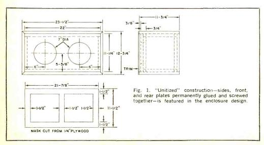
your workshop for making the beveled edges, be sure to adjust the sizes of the plates used so that the enclosure has the same inside dimensions called out in Fig. 1.
