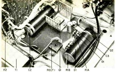
To prevent components from shorting against chassis, install spacers between the chassis and the power supply board.
