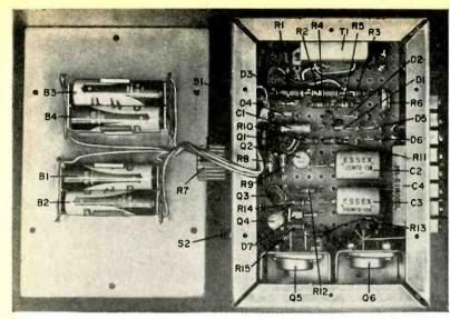
Fig. 2. In layout used by the author. much of the circuit is part of the auamplifier. a separate amplifier module is used, the blanker assembly is made smaller. Arrangement of components is not critical. The four batteries are for the noise blanker only. The amplifier requires a separate battery or a power-supply unit.
