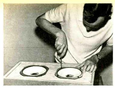
Fig. 4. T-nuts and machine screws are provided to facilitate passive radiator and loudspeaker mounting. Note that the LEST and PR8 are designed for mounting through the front of the speaker mounting board.
