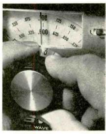
Drake SW-4A and R-4B has two separate adjustments for setting dial accuracy. Hairline can be moved by button in upper right. Skirt of tuning knob may be slipped so that 0-25 scale agrees with hairline and pointer.
