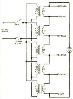
as \$1.79 each from Lafayette Radio Electronics (catalog number 99 H 6266). Wire all primary windings in parallel with each other; wire the secondaries in series in the proper phase as shown in the schematic drawing. Then, protect the setup by inserting a 1.5-ampere fuse in one of the lines of the primary circuit. Attach a line cord across the primary and an a.c. receptacle across the entire string formed by the secondaries.
