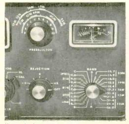
Hammarlund HQ-225 has busy-looking bandswitch because it tunes 200-kHz segments to provide extra bandspread. Control REJECTION kills heterodynes.
