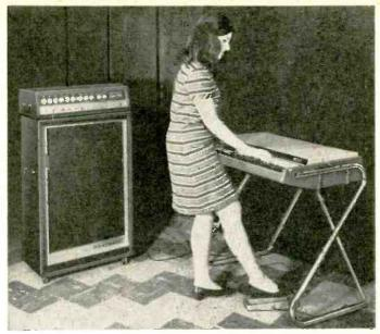
The combo organ is played standing up, using right or left foot to control volume. Organ must be fed into power amplifier. Legs are detachable and can be carried in their own case. A cover snaps over the keys and the organ becomes a second suitcase. In background is Heathkit TO-17 high-power amplifier featuring variety of inputs and speaker unit.
