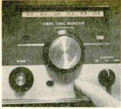
One revolution of SS-IBS dial tunes 10 kHz. Rapic frequency shifting possible with motor drive. Button on right goes up thequency, left buttom down.
