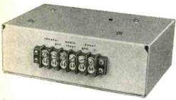
Connections to the circuit are made through a six-terminal barrier strip.
