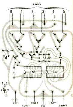
Fig. 4. Mount the components as illustrated here making sure that you orient the semiconductors properly. Note Q4 is not installed in same was as Q1-Q11.
