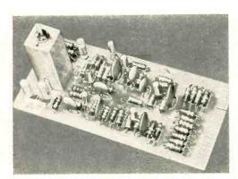
Each tone-generating board contains a basic audio oscillator and three divider circuits. Resistive matrixing between the circuits give the "Jag" its distinctive tone. Each board is slipped into place behind keyboard (see photo at right). Tuning generators is simple task.
