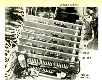
Fig. 9. Timing module and DCU circuit boards should be stacked for space conservation and neatness. Use ½"-long insulated spacers (or metal spacers and fiber washers) between each board for adequate separation. Board designations from bottom to top are M2 through M8.
