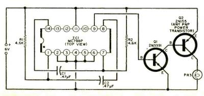
Fig. 4. This high-power modulator has a greater range than the penight version. If the lamp is mounted within a three-inch, or larger, reflector, it can be used as an intrusion warning alarm.
