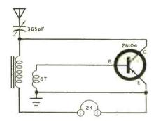
BCB loopstick with about six turns of #22 wire wound at one end of the coil. You may have to reverse the connections to the secondary winding to get best results.
