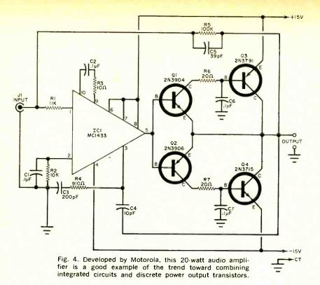
insured between the input and output stages. Small insulated heat sinks are adequate for the drivers, Q1 and Q2, but power transistor heat sinks should be provided for the output units, Q3 and Q4.
