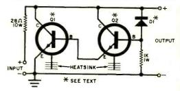
Q1, and the 2N1481 or 2N1482 for Q2. Diode D1 can be any reference diode rated at 27 volts at 1 ampere or higher—a typical one would be the 1N2954, which has a tolerance of 5%.
