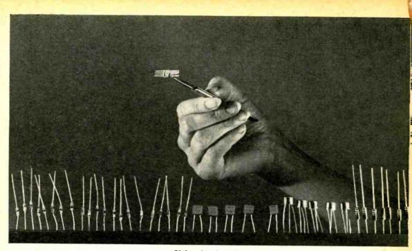
**50 functions in a single chip.** The functions of 50 separate transistors, diodes, resistors and capacitors can now be formed by the tiny dot in the center of the integrated circuit held by the tweezers.
