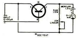
10,000-ohm potentiometer is adjusted for transistor gain variation. Beginning with a few divisions above zero, the accuracy of the microammeter will be close to 3% if the milliammeter is a 2% unit. Transistor types that can be used are: 2N408, 2N109, 2N270, or 2N407.
