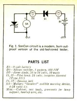
The continuity tester consists of a 9volt battery in series with a "Sonalert" module. This module is a commercially available electroacoustic device which emits a shrill audio tone when its electrical contacts are supplied with from 6 to 28 volts d.c. The power line protective circuit consists of a pair of pilot lamps, a silicon rectifier diode, and a zener diode arranged in the circuit as shown in Fig. 1.
