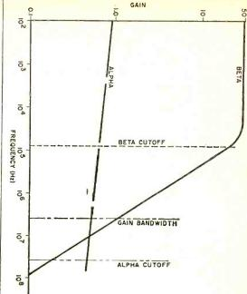
Fig. 5. This graph will help you distinguish between the various terms used to define the r.f. characteristics found in transistor specifications.
