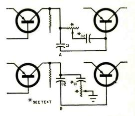
bass attenuation circuit and (b) a treble attenuation circuit. In circuit (a), the value of coupling capacitor C1 is made much smaller than normal, and C2's value can range from 1 to 25  $\mu$ F. The potentiometer value can vary from 2000 to 25,000 ohms. In circuit (b), C2 is the normal value, but C1's value can range from 0.02 to 1  $\mu$ F. The potentiometer for circuit (b) can be in the 3000- to 75,000-ohm range.
