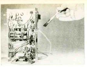
Restoration begins with a thorough cleaning of the chassis, using a small brush and/or vacuum cleaner. Stubborn dirt, grease, and capacitor electrolyte are easily removed with carbon tetrachloride—pitch with kerosene or benzene. While cleaning the chassis, be on the lookout for heat-scarred and broken components, frayed wires, and cold solder connections.
