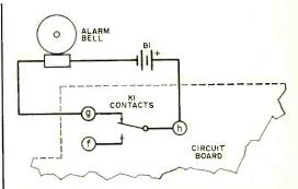
Fig. 5. A remote bell, or other alarm, with its associated battery power can be connected as shown here.
