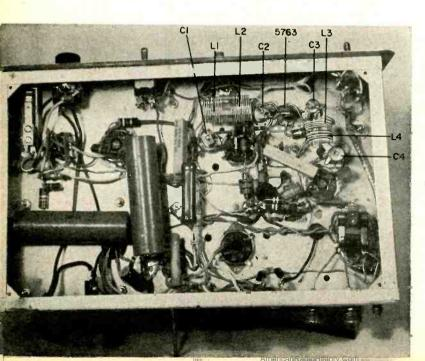
Fig. 2. The new circuit installed in the author's Globe Scout transmitter, replacing the original oscillator bandchanging components and output network.
