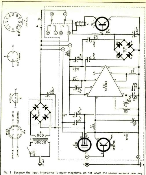
source of r.f. noise, as operational range will be reduced. The metal antenna can be any shape desired.
