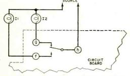
Fig. 6. When someone approaches the sensor antenna, 11 goes off while 12 comes on. This signaling can be used in a number of ways, as explained in text.
