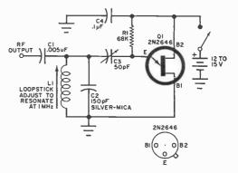
The UJT operates at submultiple of output frequency and shock-excites tank circuit to generate r.f. output. This oscillator circuit can reach 1.5 MHz.
