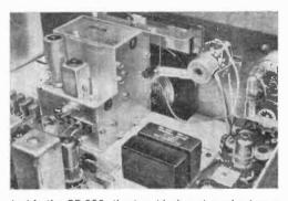
Inside the SB-310, the two black rectangular boxes are the special filters that permit optimum selectivity on both international broadcast and ham bands. Tunable linear oscillator is at upper left.
