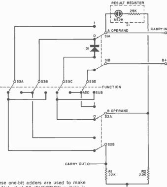
Fig. 2. Five of these one-bit adders are used to make the Binary Adder. Note that S3 (FUNCTION switch) is common to all five stages. Readout is via neon lamps.
