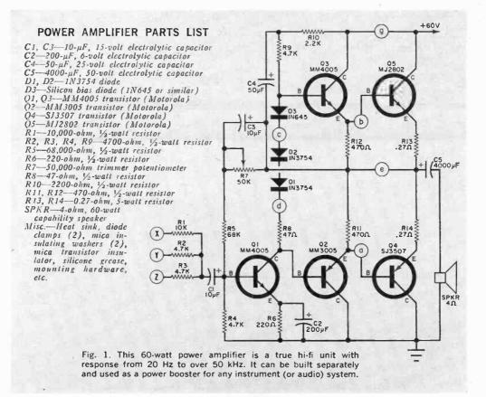
fier that provides exceptionally clean output at high power and low cost. The first stage, Q1, is a conventional voltage amplifier.
