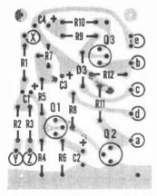
serving that a red dot on each diode case identifies the cathode of the diode. Failure to wire these diodes correctly may damage the power transistors.
