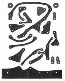
Fig. 2. Actual-size printed board for amplifier. The two power transistors and associated components are mounted externally due to their heat dissipation.
