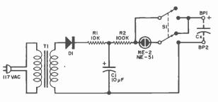
Fig. 2. Reader Eugene Richardson's capacitor tester has visual readout.
