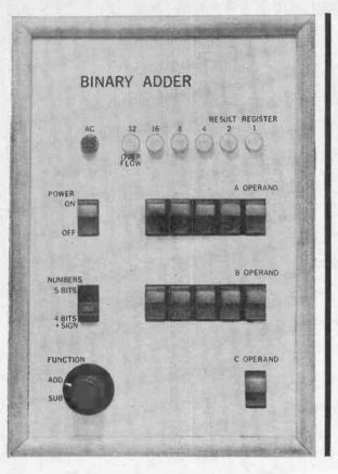
DEMONSTRATING BINARY COMPUTATION WITH THE Binary Adder
