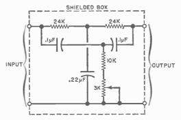
series with the signal lead and adjust the potentiometer for maximum 60-Hz rejection.
