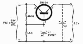
equal to  $C_f H_{\rm FE}$  where  $H_{\rm FE}$  is the current gain of the transistor being used. In the example shown, the effective  $C_{\rm F}$  is about 25,-000  $\mu$ F.
