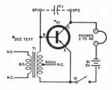
Fig. 1. Suggested by Kenneth Scharf, this capacitor tester has an audio output tone whose frequency is determined by the capacitor undergoing test.
