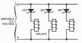
voltage goes up, each zener will conduct at its voltage and close its associated relay. You can select the zeners and relays for almost any range of d.c. voltage required.
