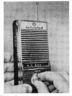
Volunteer firemen or auxiliary police should welcome the advantages of a desk or bedside VHF receiver. Sensitivity with built-in antenna is usually sufficient for local 3-7 mile VHF reception. Use of outdoor antenna tuned to VHF will triple receiving range. Similar models tune CB or aero bands.
