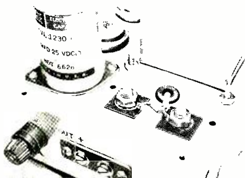
Output side of the chassis showing diode installation, power output terminals, filter capacitor C3 , and output fuse F2 .
