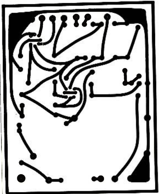
Fig. 5. Actual-size layout of PC board. Drill as shown in Fig. 2; mount components as per Fig. 3.
