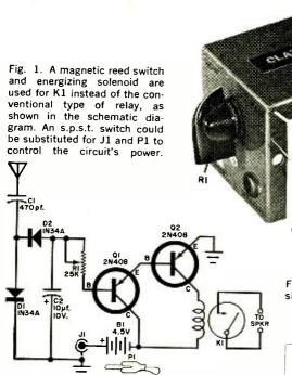
Parts layout and placement are not critical, but keep component leads as short as possible and neatly dressed.
