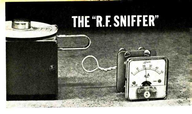
NO HAM OR CB'ER should be without some type of r.f. signal indicator for trouble-shooting and operating transmitters, r.f. amplifiers, and oscillators. A simple r.f. field strength meter fits the bill nicely. This device is almost as versatile in r.f. circuits as a multimeter is in d.c. and low-frequency a.c. circuits. Furthermore, it is easier to use and it is more compact than most multimeters.
