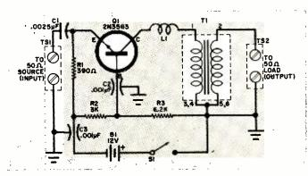
Fig. 3. One of several experimental circuits presented in Vari-L's Application Bulletin 167, this amplifier is said to furnish gains up to 10 dB over a frequency range of 1 to 300 MHz.
