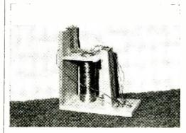
is a 12.5-volt model. It works just as any other relay does, but is about 50 times as large. One perforated metal strip serves as the armature, and the other as the stationary contact.
