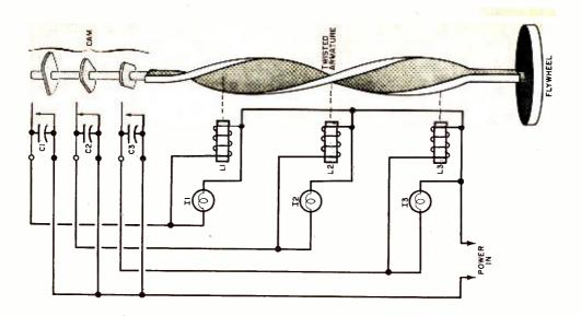
Fig. 1. Each of the cams on the twisted armature is related to a respective electromagnet to pulse the power at a precise time in order to generate maximum torque and speed while the armature is rotating.
