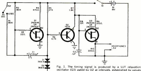
oscillator (Q3) gated by Q2 at intervals, established by values chosen for resistors R1 and R2 and capacitor C1, and by Q1.
