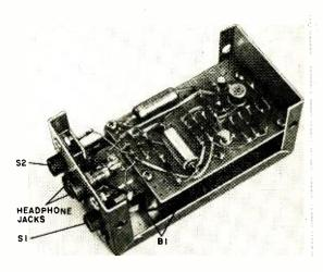
The two series-connected 9-volt batteries comprising B1 are tucked away under the circuit board. The headphone jacks and switches are panel-mounted.
