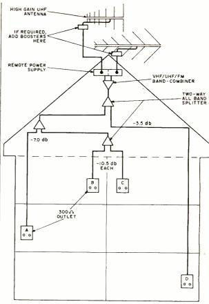
Balancing a system for proper distribution of signal strength is not difficult. Outlet D, being at the end of a long run, can be tapped off near the head end and be fired with about 50% of the total signal, whereas the line feeding outlets B and C receives only about 10% of the total signal yet delivers essentially the same amount of signal to the TV set as outlet D. How much signal you need depends upon the system's losses. Work with dB's.
