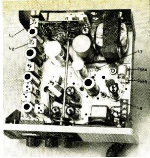
Fig. 13. No part changes are required to convert the receiver section of the Lafayette HE-20D transceiver, but three components have to be replaced or modified to put the transmitter on 10 meters.
