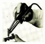
action on the rubber bulb lifts the solder by vacuum from the connection. The tip's 360° coverage plus capillary action of the solder is said to result in a perfect resoldered connection. Tips come in five sizes.
