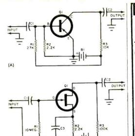
Fig. 4. A VOM of relatively low input resistance can be used to measure the base-emitter voltage of a bipolar transistor (A) without excessive circuit loading. However, the same VOM would act as a virtual short circuit if used in a similar manner to measure the source-gate voltage of a FET (B).
