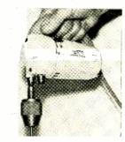
be used with ¼" drills is the most convenient and inexpensive type. Many hardware stores sell imported chucks for about 98 cents. The mixer-cum-drill can then be used to drill holes in metal chassis or woodwork. You can also take advantage of the variable speeds available on this type of mixer.
