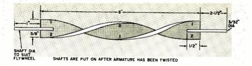
Fig. 4. The lengths of the shafts on each end of the soft iron armature should be long enough to accommodate the flywheel on one end 1/2"DIA 3/32"DIA (about 1"), and the cams and spacers on the other end (about  $2\frac{1}{2}$ ").
