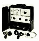
CR-35 checks gas, emission, shorts, opens, grid cutoff, and cathode life. It also rejuvenates, repairs shorts, and determines boosteffective-61. ness. Continuously variable, meter - monitored test voltages assure the availability of
