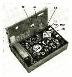
Spread FM oscillator coil L3 as much as possible without breaking or shorting any components. Shift the FM broadcast band as far down as it will go by adjusting C2. Tune in a station at about 150 MHz and adjust C1 for maximum volume. There is no need to make any other adjustments in the receiver.
