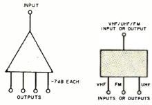
Signal splitters, multiple set couplers and amplifiers are usually schematically represented by triangles, squares, and rectangles, but not by circles.
