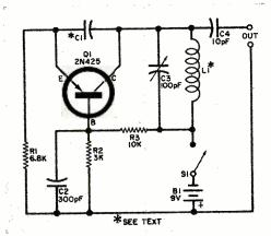
dary winding of a small 455-kHz transistortype i.f. transformer. Capacitor C1 is a gimmick made of two 1-inch pieces of No. 20 cotton-covered wire twisted together. You can try a small 25-pF capacitor instead of the gimmick, if you wish. The leads should be twisted just enough to furnish a small amount of feedback and stable operation.
