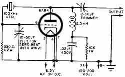
accompanying diagram. Besides satisfying the requirements you set forth, this circuit will give you a hefty signal. The 6AB4 tube does a good job, but almost any triode tube can be used instead: To operate, plug in a 100-kHz crystal and connect the output of the calibrator to the antenna input of your receiver.
