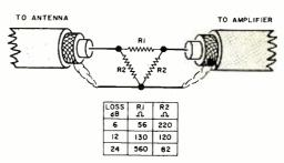
Simple resistive pads for 300-ohm line (top) and for 75-ohm coax cable (bottom) can be assembled to cut signal strength and maintain correct impedance.
