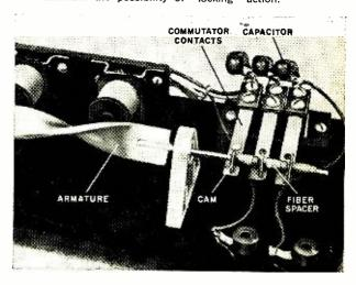
The armature is fabricated from a  $\frac{5}{8}$ "wide x 6"-long strip of 1/8"-thick soft iron twisted as shown in Fig. 4; aluminum or other non-ferrous metal cannot be used. You can start with a strip about 2' long. Put one end in a vise and attach a long wrench on the other end. Twist the strip until you wind up with 1 complete revolution (360°) within a 6" length. Mark this piece off and use a hacksaw to cut away the unused portions. Cut a notch on each end as shown.
