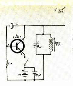
value of the resistor must be adjusted to suit the transistor—try a nominal value of 47,000 ohms; it will never be less than 10,000 ohms and rarely more than 75,000 ohms.
