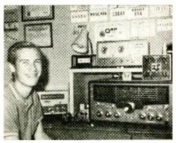
Steve Buerg, WN6THT, Daly City, Calif., made 458 contacts in 46 states and five continents in two months. How's that for a record? A Hallicrafters HT-40 transmitter and SX-101 receiver and a Hy-Gain 14-AVS vertical antenna are his tools. HAM A RECEIVER
